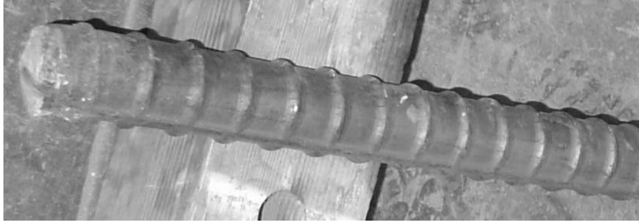
Figure 2.2: Bamboo ribs on a #18 bar
