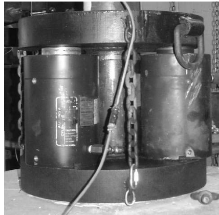
Figure 2.7: Triple ram used to yield and fracture #18 bars
