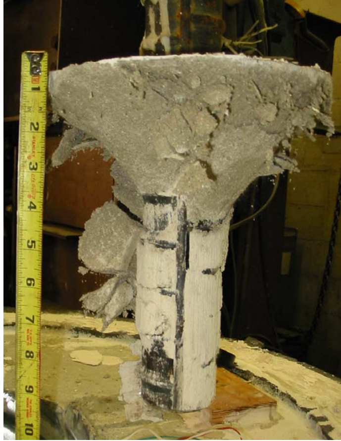
Figure 4.10: Grout cone and sheared grout: 18F04
