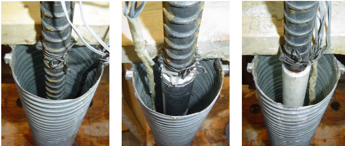
Figure D-2: Anchorage conditions in each specimen - AD8-FB (left), AD8-D1 (center), and AD8-D2 (right)
