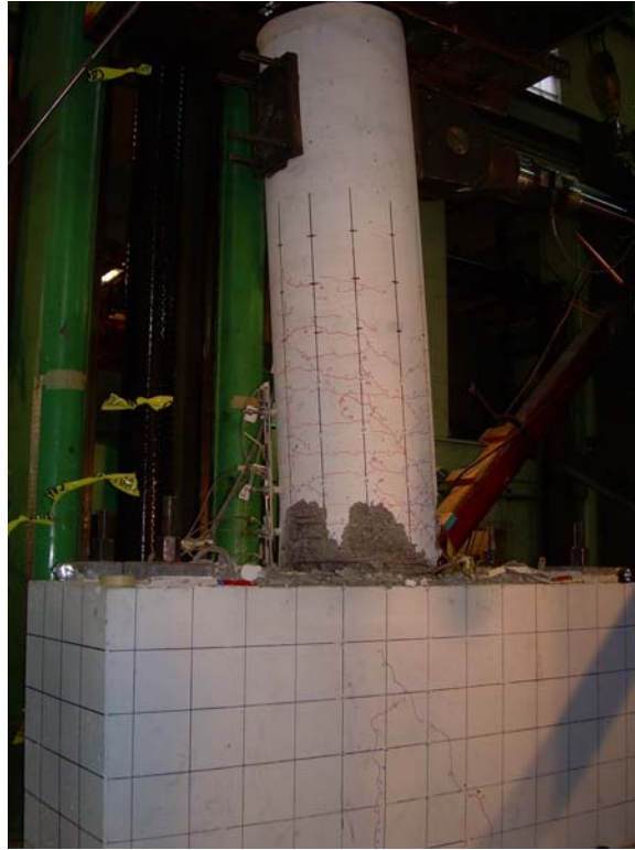
Figure 4-41: Specimen LB8-D1 displaced during Cycle 34 (7.20%/-7.06%)
