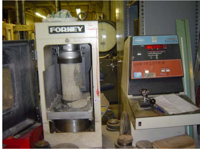
Figure B-11: Compression testing of a 6-inch by 12-inch cylinder
