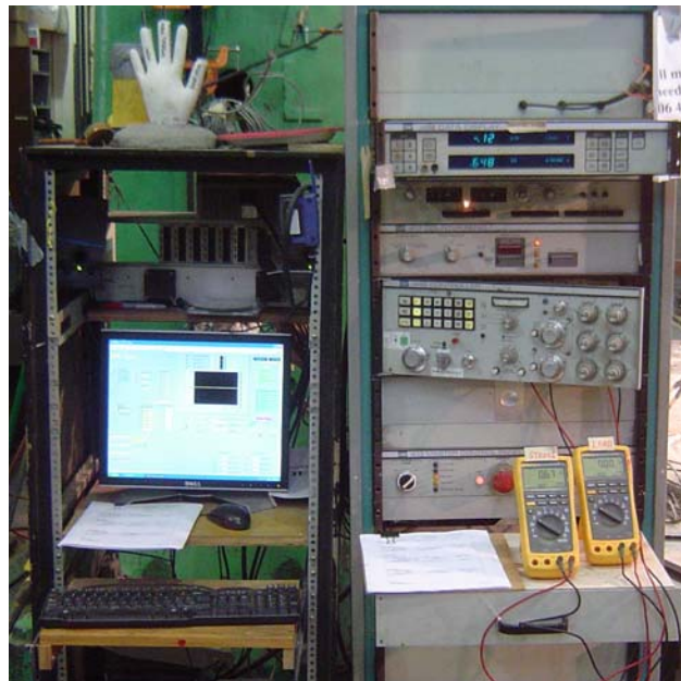
Figure 3-5: Data acquisition system and MTS controller
