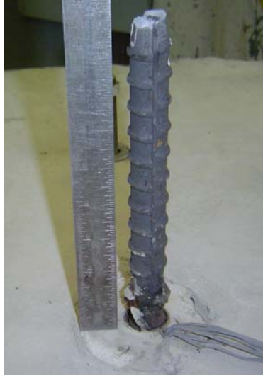
Figure D-13: Fractured bar in Specimen AD8-D2
