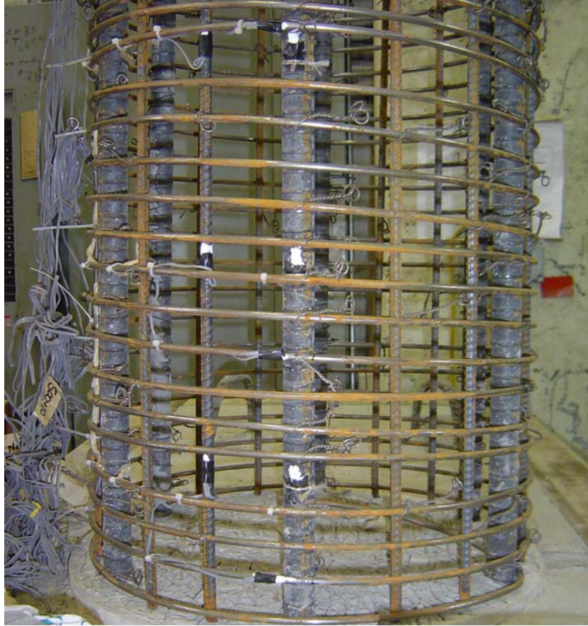
Figure 3-12: Strain gages located in the column
