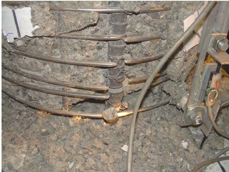
Figure 4-40: Bar 4 fractured in Specimen LB8-D1 during Cycle 34 (7.20%/-7.06%)
