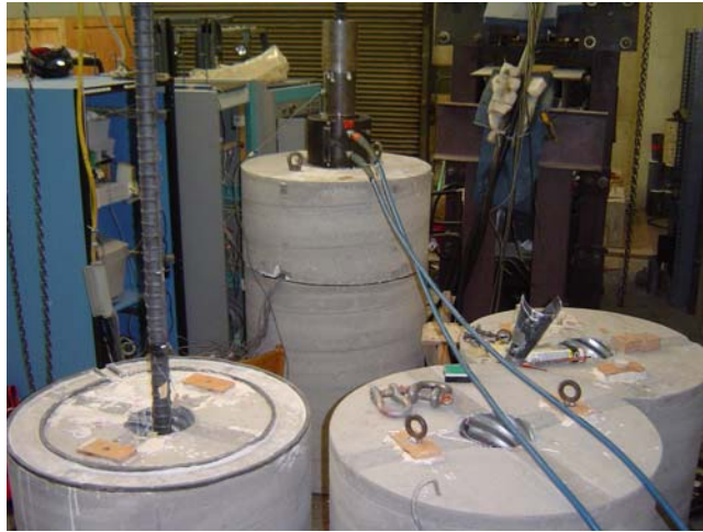
Figure 1-5: Full-scale pullout test set-up
