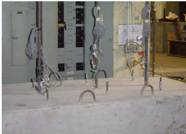
Figure D-5: Pullout test specimens
