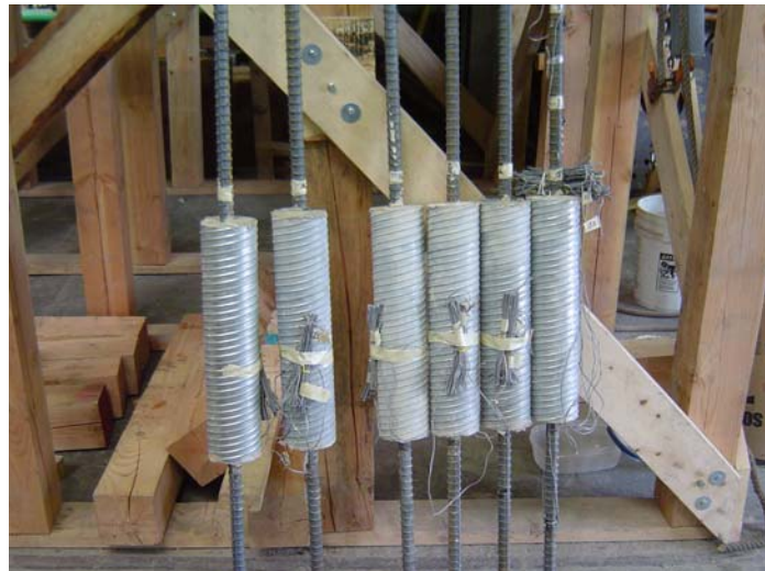
Figure B-26: Ducts grouted onto the column bars for LB8-FB
