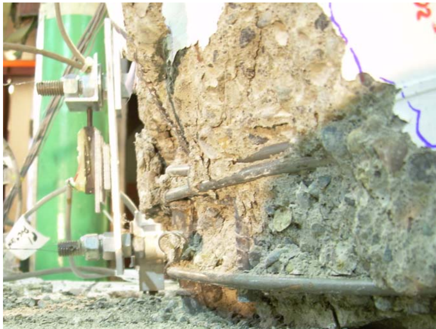
Figure 4-36: Bar 1 buckling in Specimen LB8-D1 during Cycle 32 (5.77%/-5.67%)
