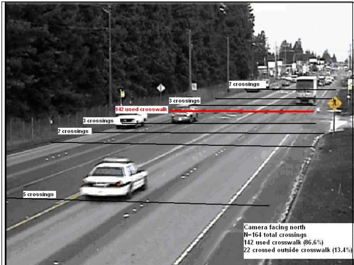
Figure B-8. Pedestrian crossing paths to the north of S. 180 th Street— before condition (Spanaway) (Kopf and Hallenbeck 2005)
