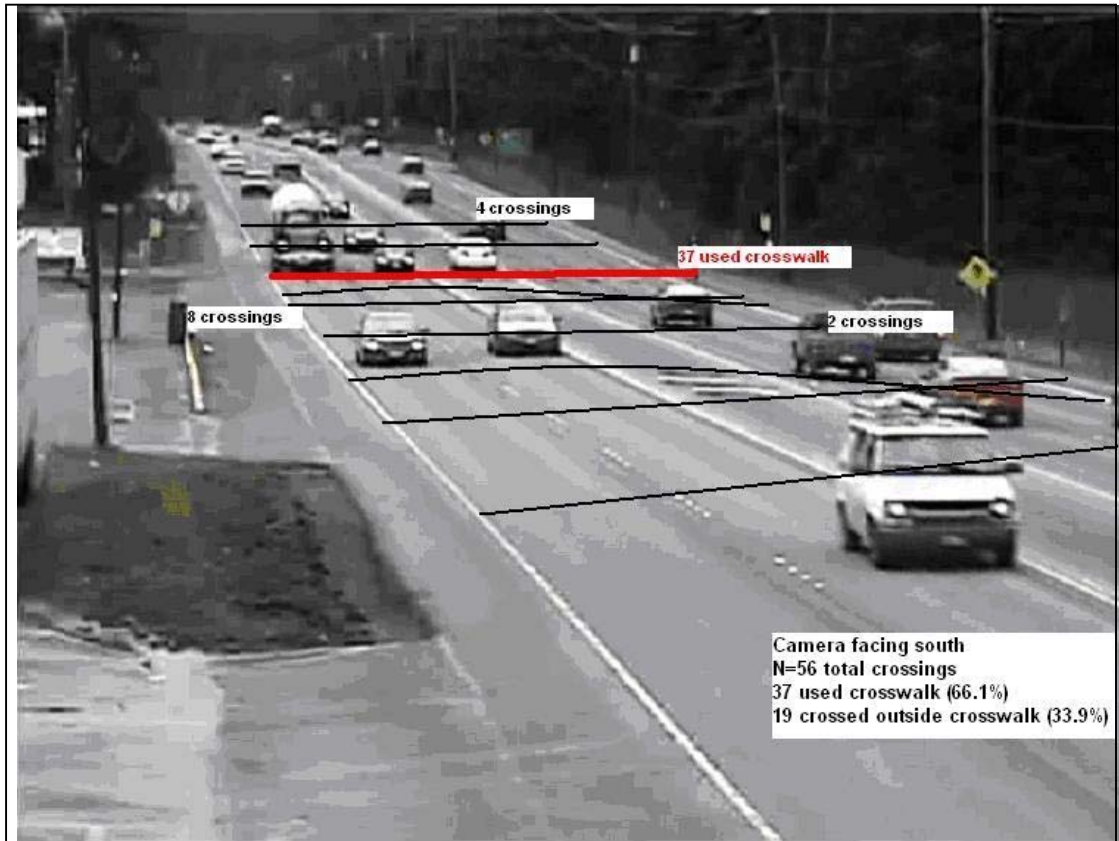
Figure B-9. Pedestrian crossing paths to the south of S. 180 th Street—before condition (Spanaway) (Kopf and Hallenbeck 2005)
