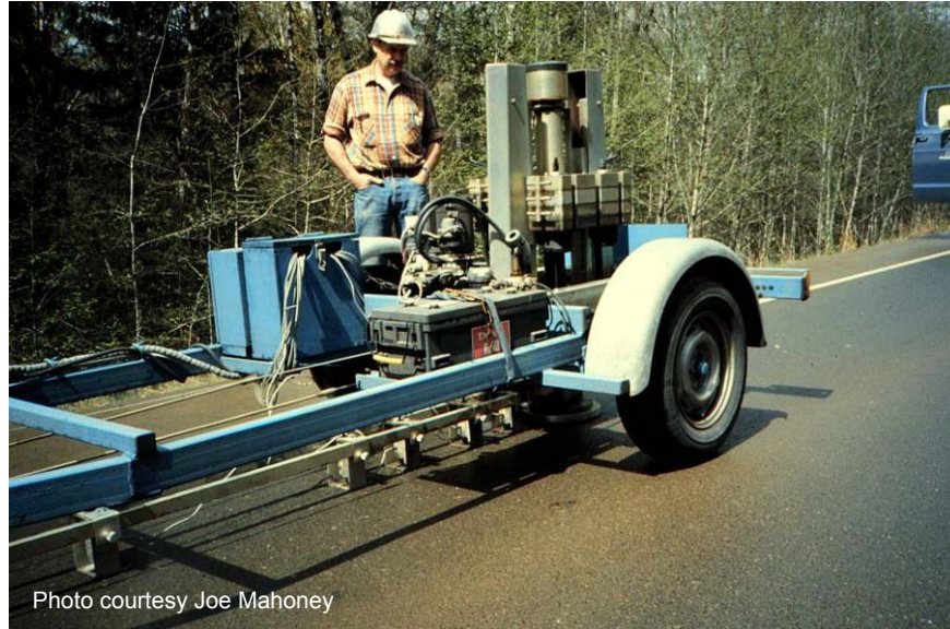
Figure 9 Falling weight deflectometer (FWD).
