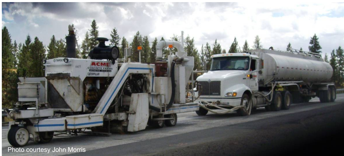
Figure A-81. Diamond grinding equipment.
