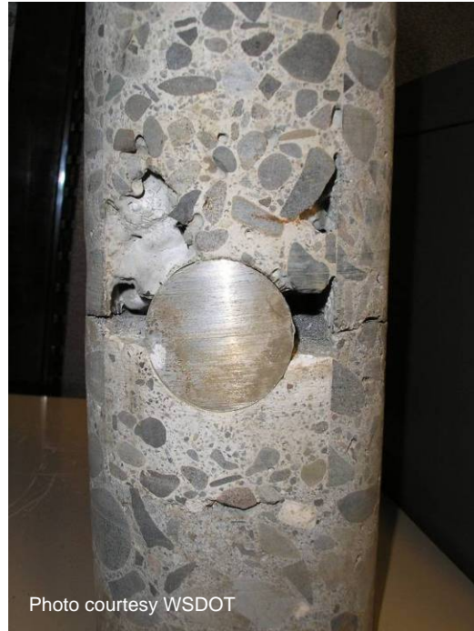
Figure A-70. Poor consolidation.
