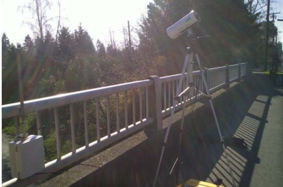
Figure 4-1: a) Selected freeway test corridor on SR 520. b) Bluetooth sensor (left) and portable ALPR (right) used to collect travel time data at the 24 th Ave location.
