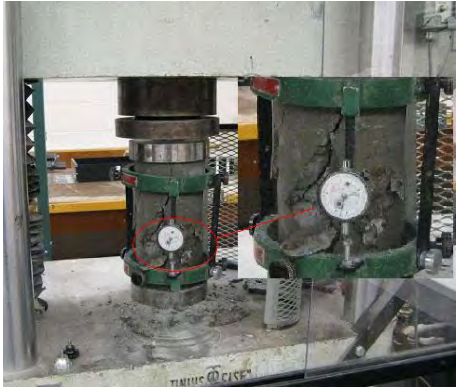
Figure 3.3 Compressive and Modulus of Elasticity Test
