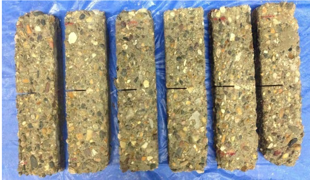
(c) Samples after 1,500 F/T cycles.
