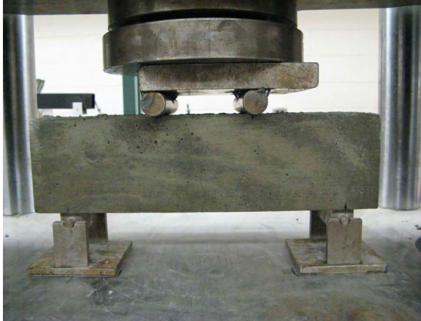
Figure 3.4 Flexural Strength Test
