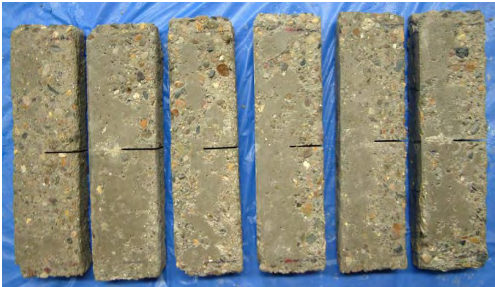
(b) Samples after 900 F/T cycles
