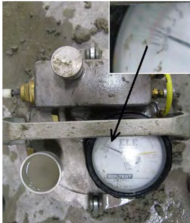
Figure 3.2 Air Content Test
