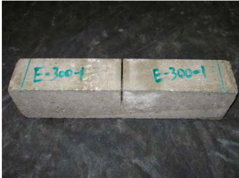
(b) Notched sample cut by diamond saw
