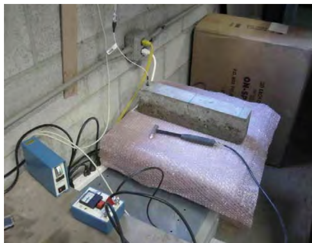
(b) Thick pad support approach used in this study
