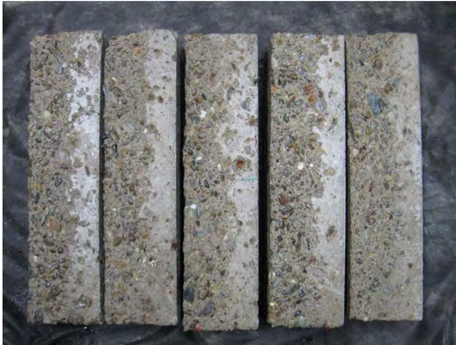
Figure 4.1 Surface Scaling of Concrete Samples with LD-WSDOT Aggregate Sources at 1,500 F/T Cycles.
