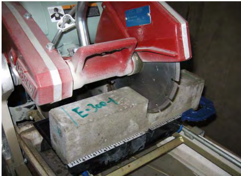
(a) Notch-cutting by diamond saw
