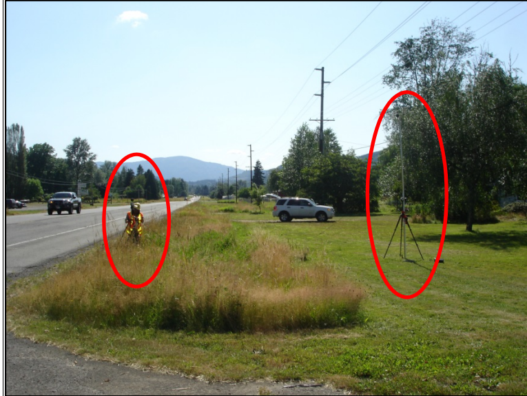
Figure 10: Sound level meters at a test site on US 12
