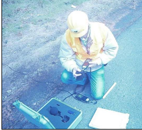
Figure 9: Verifying calibration of Type 1 sound level meters before measurements.
