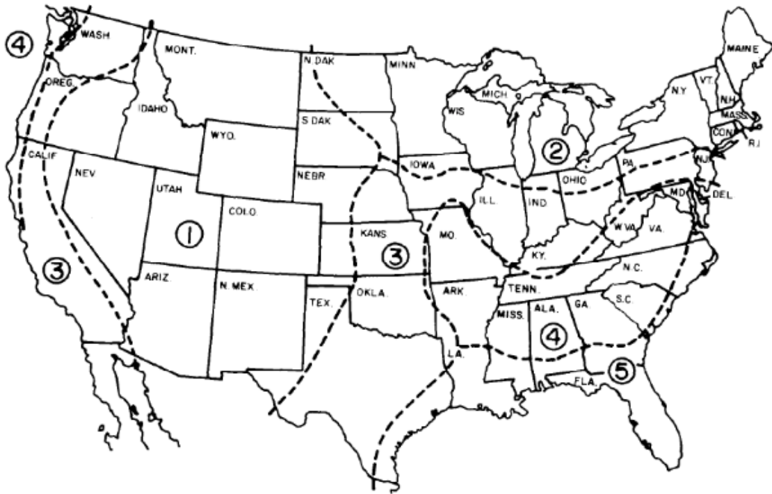
Figure 2. Decay severity zones for wood poles, ranging from the least severe decay conditions in zone 1 to the most severe decay conditions in zone 5 (USDA 2013).
