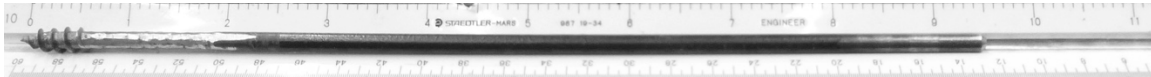
Figure 18. Drill bit used for checking decay. The total modified bit length was 9.5 inches. The bit was created from a FastenMaster® HeadLok® HLG M010 heavy duty flathead fastener. The head was removed and the threads were machined down to four full turns, starting at the tip.
