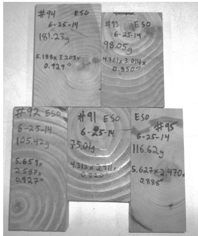
Figure 7. Example moisture content samples. The pictured samples have been trimmed to remove the outer treated areas but they have not been oven-dried.
