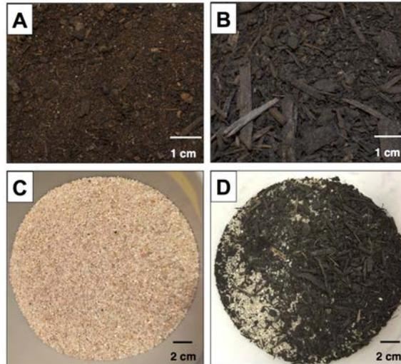
**Figure 2:** *Bioretention soil mix used in the experiment. (A) Silver Springs compost; (B) Royal Classics compost; (C) coarse sand; (D) bioretention mix after mixing compost with sand at a 40:60 volume ratio (Silver Springs compost).*
