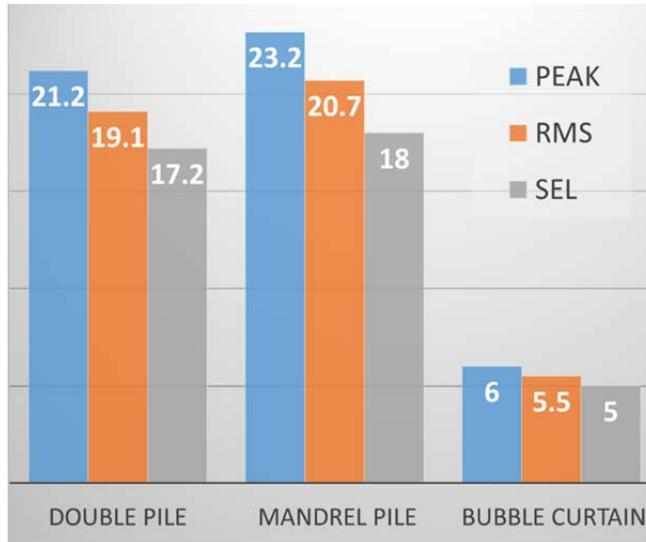
**Figure 29:** Summary of the results of the acoustic measurements in dB
