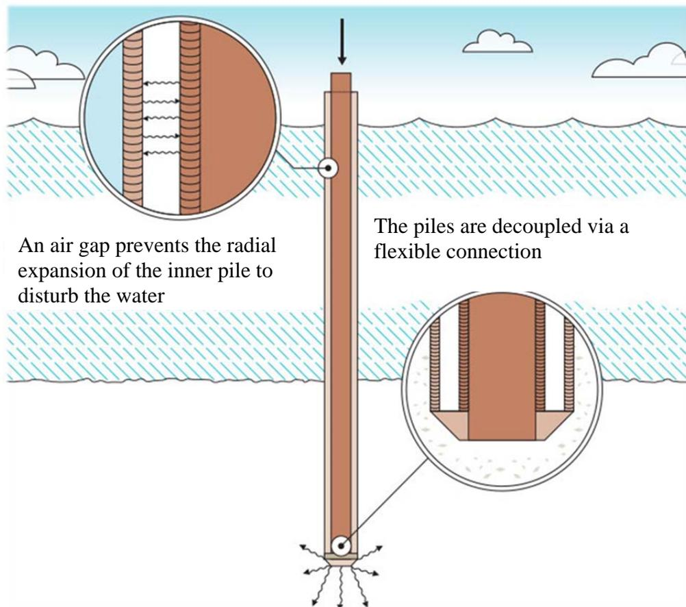
**Figure 5:** Schematic of the double wall pile
