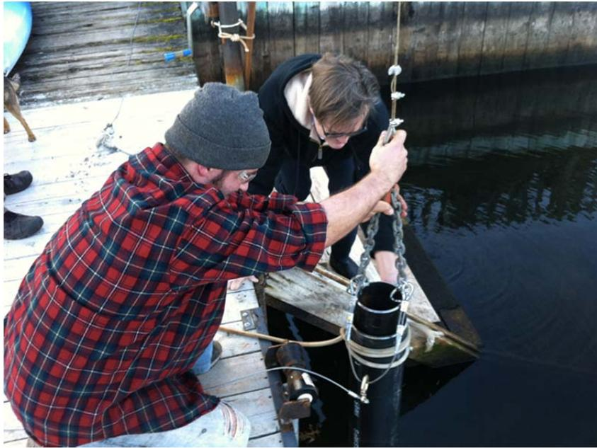
**Figure 8:** A subscale pile being prepared for testing
