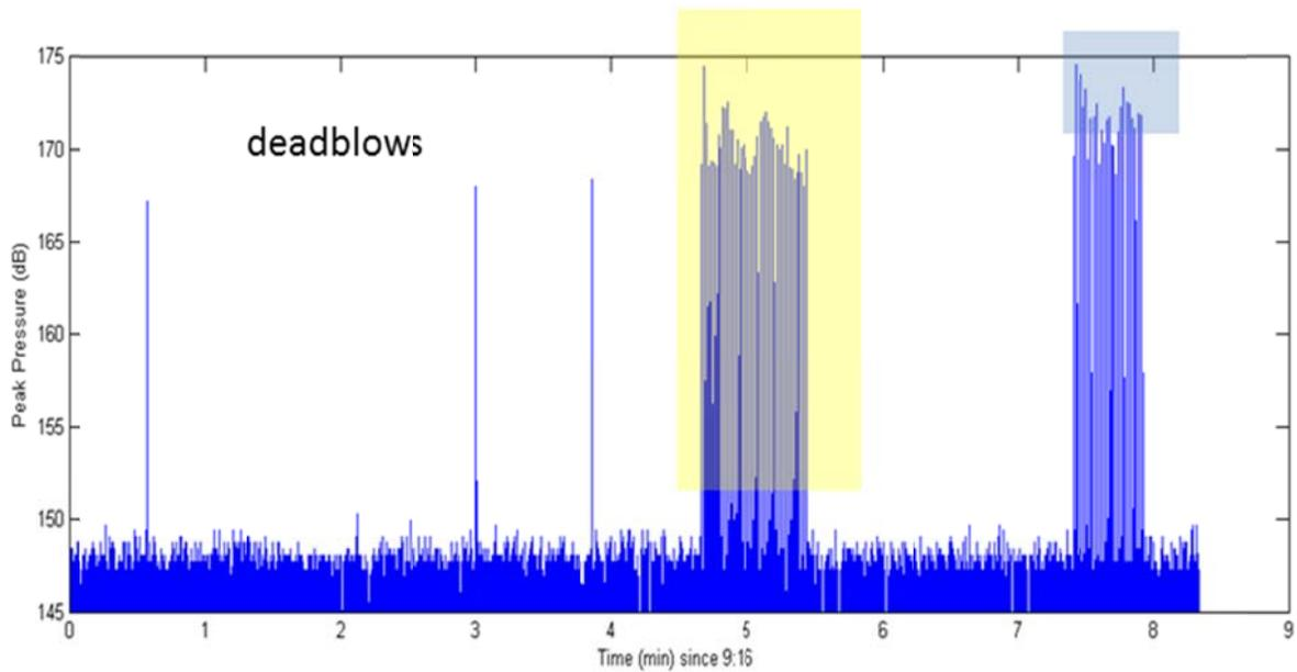
**Figure 13. Pressure recording from the autonomous system at range 135 m on all hammer strikes made during mandrel wall pile test on October 30<sup>th</sup>. Starting at approximately minute 4.5 on this scale fuel settings were changed in an unknown manner and duration causing the modulation shown in yellow shade. The blue shade denotes the period where fuel setting was definitively set to and held at constant setting = 4. NOTE: pressure is absolute pressure expressed in dB re 1  $\mu$ Pa.**
