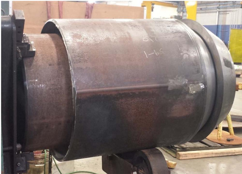
**Figure 14:** Complete double pile shoe
