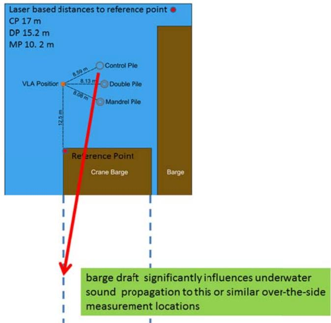
**Figure 8. Showing potential issues relating to the underwater sound measurements taken over-the-side of the Crane Barge at the approximate location given by the red arrow head. The crane barge extends beyond the brown-colored area as shown by the dotted lines. The draft of the barge significantly influences underwater sound propagation in the direction of the red arrow. The influence depends on the particular pile under test.**
