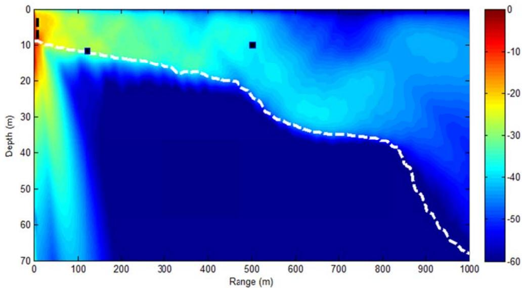
**Figure 22. Notional field strength in decibels for SEL (i.e., proportional to) from impact pile driving based approximately bathymetry (white dashed line) for the Tacoma site and tidal conditions in effect at 1300 on October 29<sup>th</sup>. The black marks show approximate locations of the vertical line array near range 8 m, and the two remote measurements at ranges 122 m and 502 m.**
