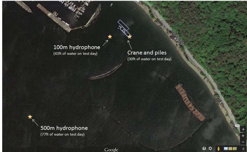
**Figure 24:** Placement of the far-field hydrophones
