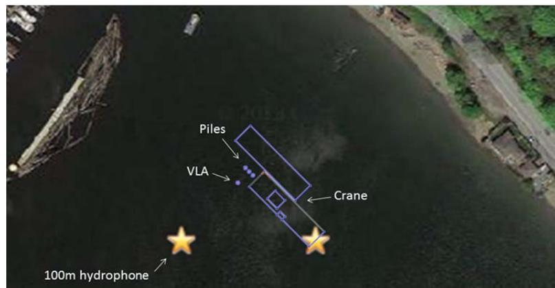
**Figure 23:** Placement of the near-field hydrophones
