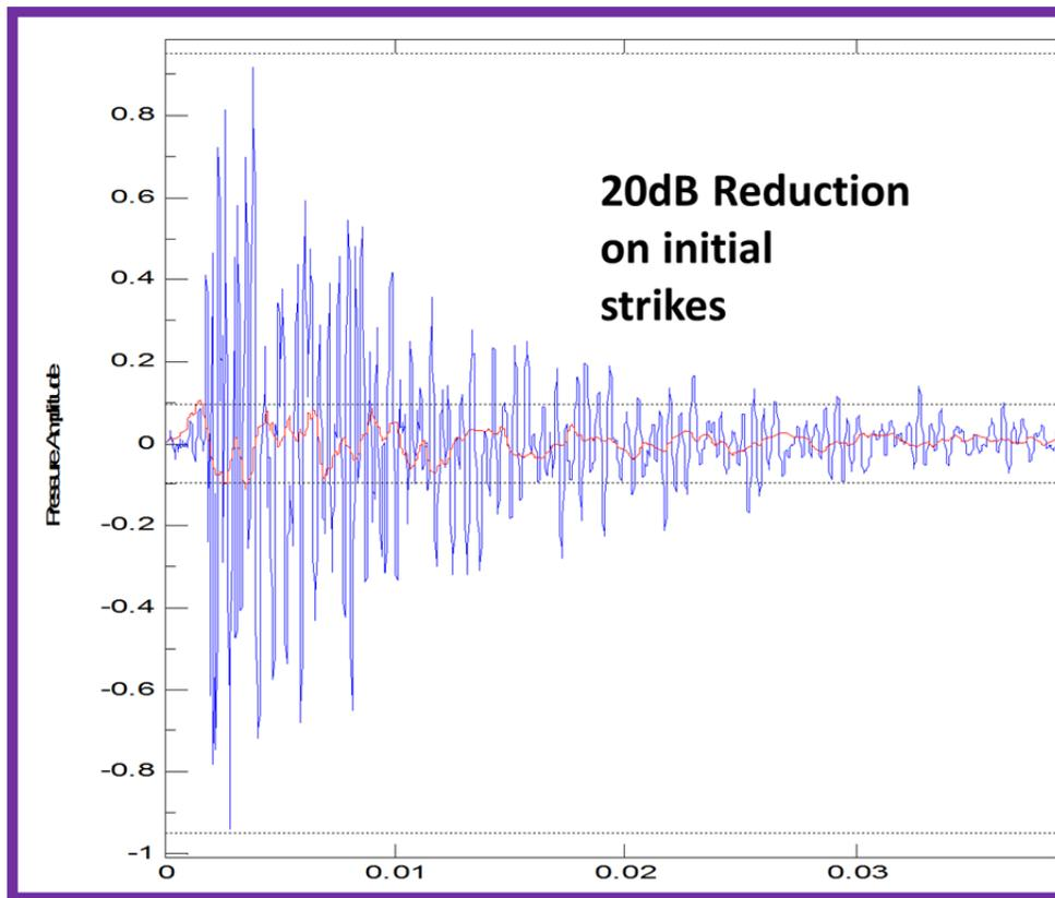
**Figure 10:**  $p(t)$  pile signals overlaid and magnified
