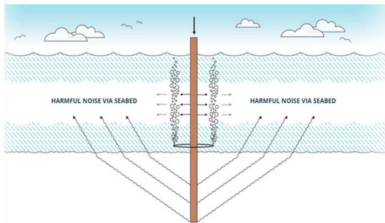
**Figure 1:** Illustration of how sound from the seabed is transmitted unhindered by a sound shield surrounding the pile in the water, e.g., a bubble curtain.
