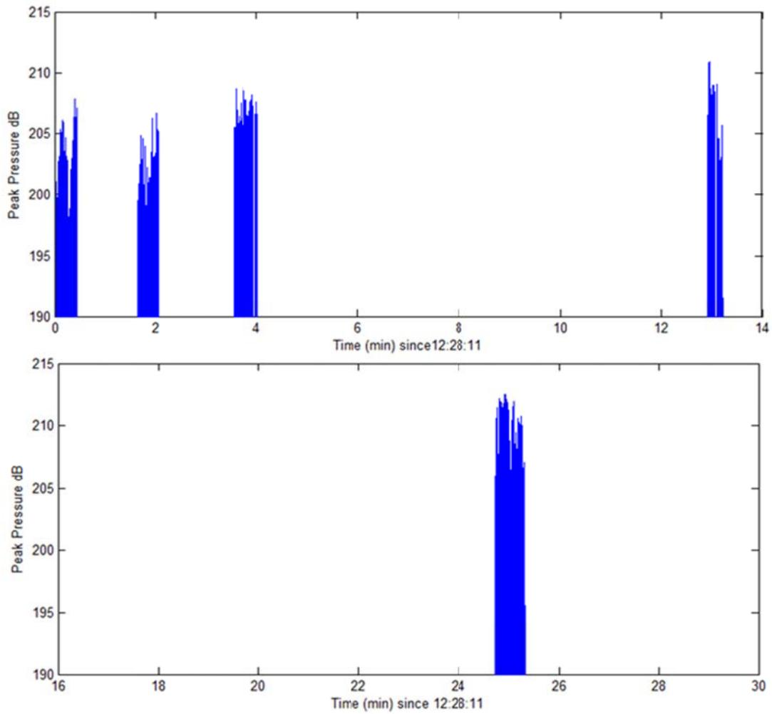
**Figure 10. Pressure recording from channel 9 (lowest channel) of the VLA for series of hammer strikes made on the control pile on October 29<sup>th</sup>. Upper plot shows period during which the hammer fuel setting was changed and/or the bubble curtain was activated and deactivated. Lower plot shows final set of strikes during which the hammer fuel setting was held constant at setting = 4. Data are absolute pressure expressed in dB re 1  $\mu$ Pa.**
