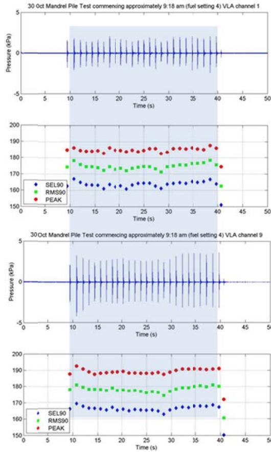
Figure 17. Channels 1 and 9 of the VLA corresponding to the October 30<sup>th</sup> series of tests involving the mandrel pile. This data is compared with control pile data shown in left column of Fig. 15. Data from shaded areas used in the comparison.
