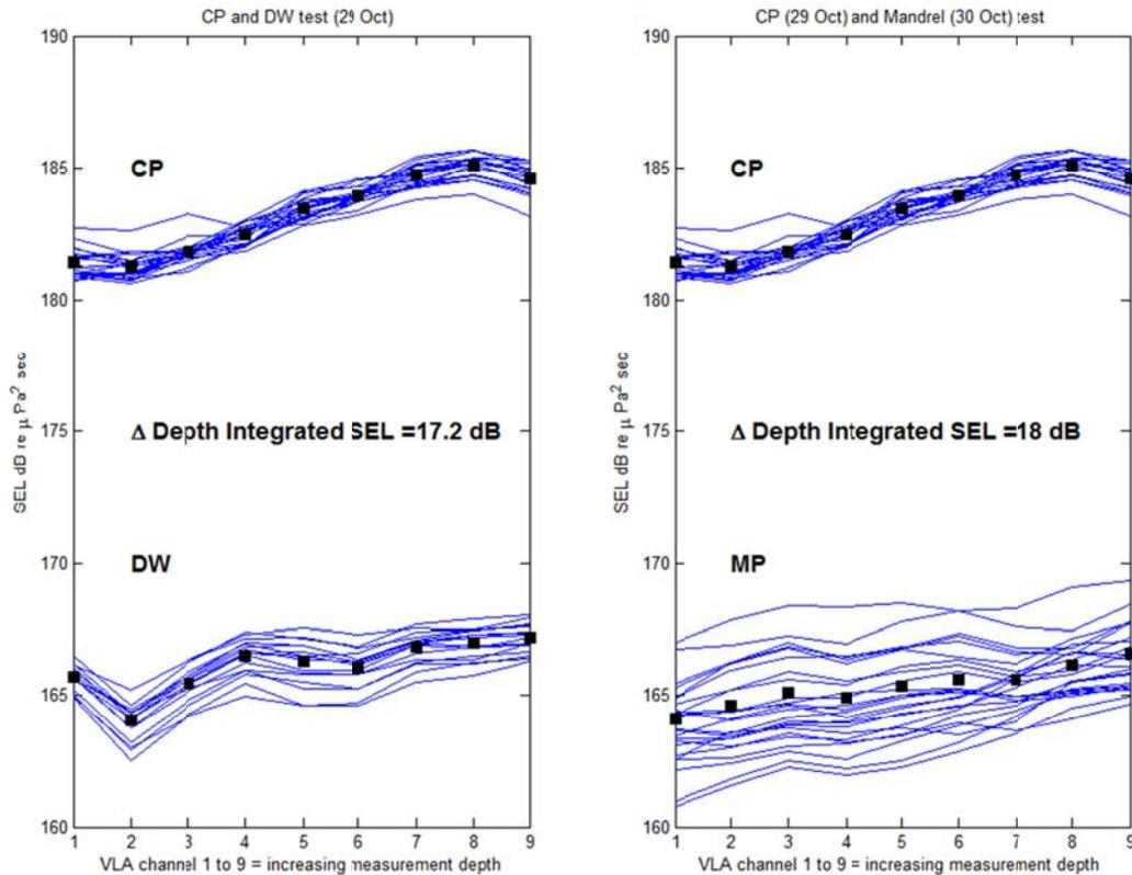
**Figure 19. SEL as a function of hydrophone channel for individual strikes (thin blue lines) for the control pile (CP), double wall test pile (DW) and mandrel test pile (MP). Black squares denote the linear average of individual strike SEL for each hydrophone. These data are then summed over all hydrophones (in linear space) with the result decibel difference shown for each test (17.2 dB for the DW test, and 18 dB for the MP test).**
