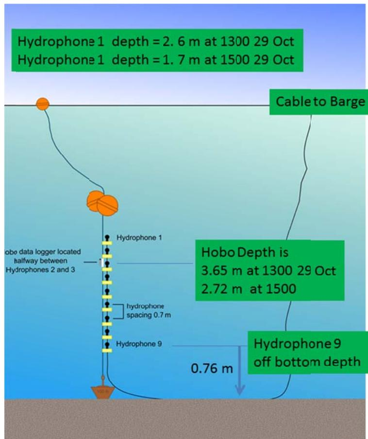
**Figure 4. Position of the 9 hydrophones on the VLA with respect to depth. Note this relation changes according to tidal conditions. Tidal elevation 0900-0930, 30 October is similar to that at 1300 29 October.**
