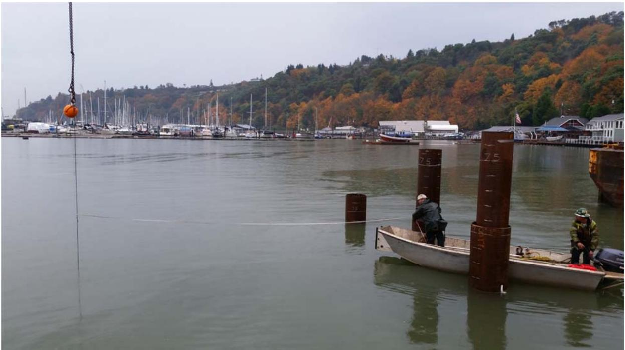
**Figure 3b.** Photograph made on October 30<sup>th</sup> of the 3 piles shown in order of nearest to farthest: Mandrel Pile, Double Pile and Control Pile. The VLA, now under tension is shown on the left while its range from the piles is measured.
