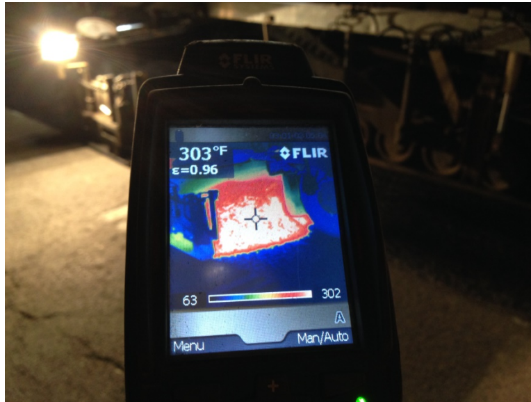
Figure B1.2 WMA over 300°F in Paver Screed
