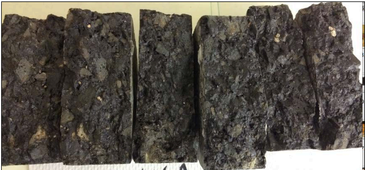
Figure B2.9 HMA Samples after IDT Thermal Cracking Tests
