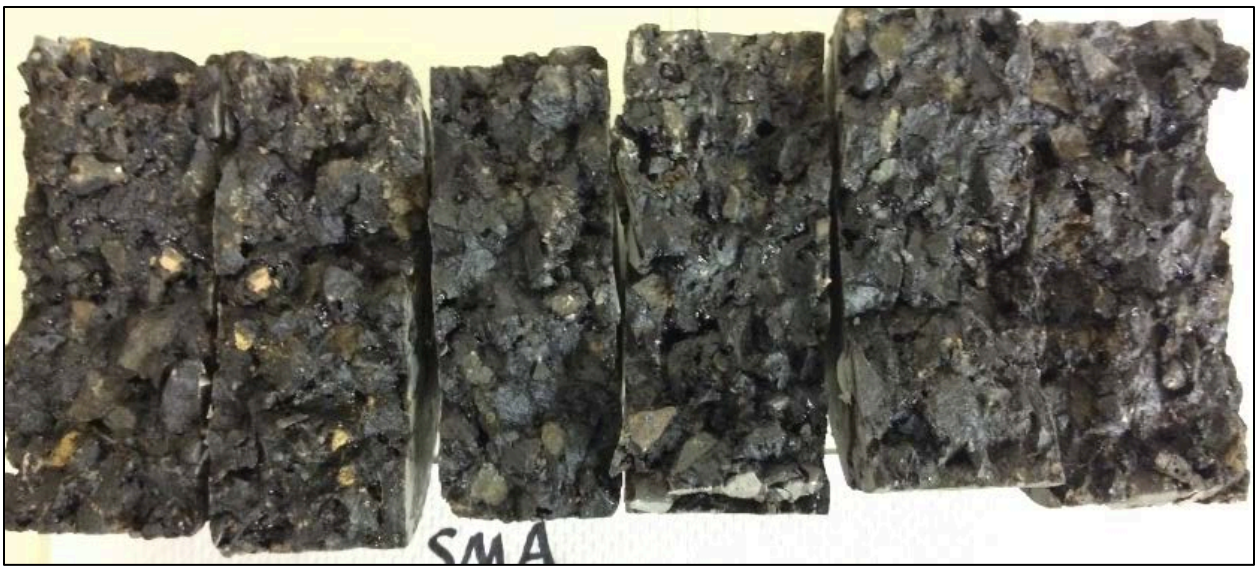
Figure B2.4 HMA Samples after IDT Fatigue Test
