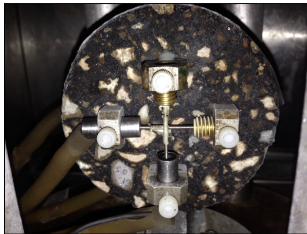
Figure B.3 Asphalt Mixture Sample Mounted with LVDTs
