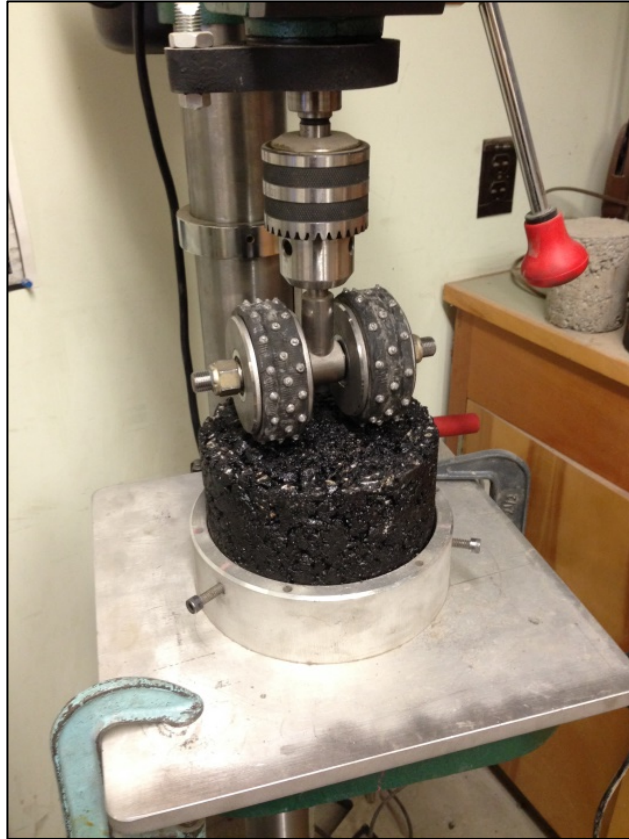
Figure B.145 Studded Tire Wear Simulator with Gyrotory Sample
