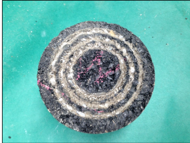
Figure B.2 Field Core Sample after Studded Tire Simulation
