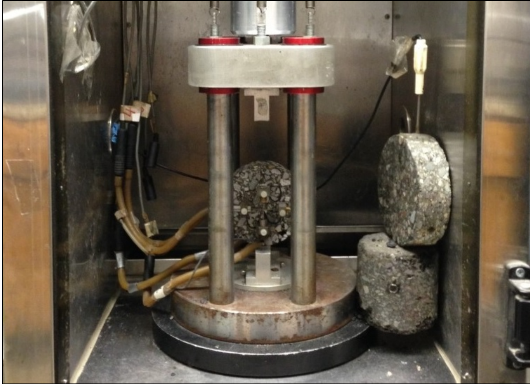
Figure B.4 IDT Test Machine Setup
