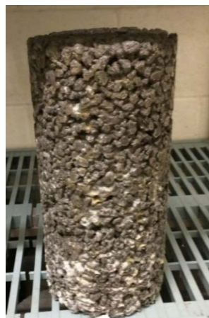
Figure 18- Specimen from curing 1A3M at 28-day age, with white stains of leached materials.
