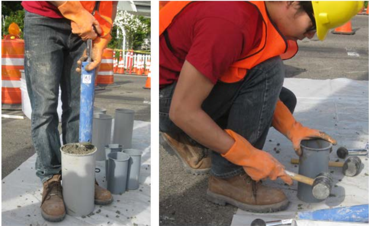
Figure 9- Compacting PC into cylindrical specimens: (left) by the Proctor Hammer, (right) additional strikes of the mallet to avoid undesired pockets of air.
