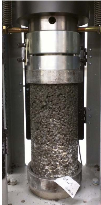
Figure 10- Compressive strength test experimental setup.
