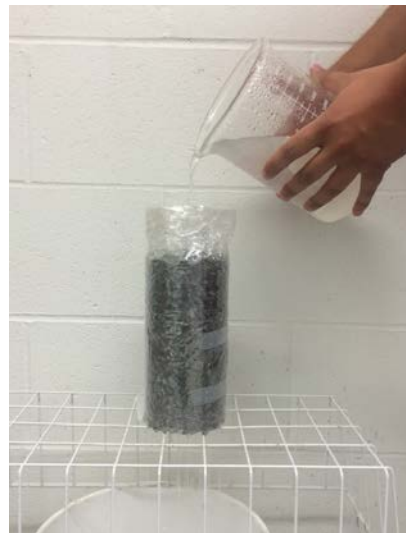
Figure 2- Infiltration test setup.
