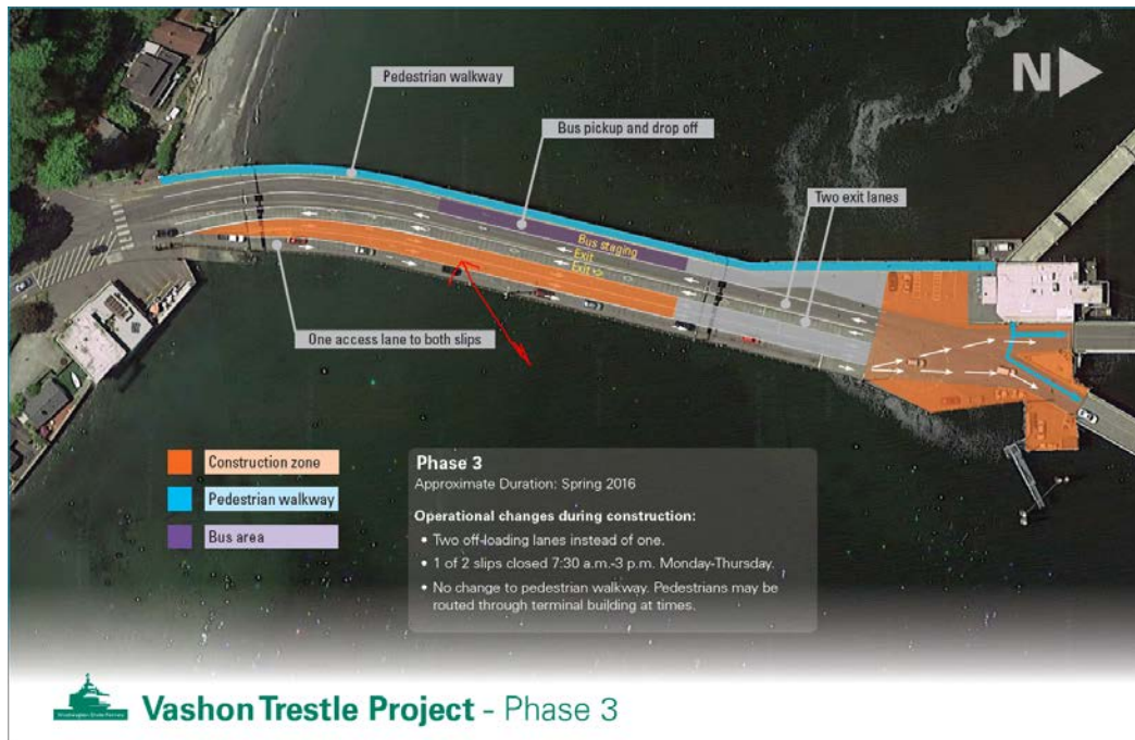
Figure 4- Vashon Ferry Terminal Construction Lanes (WSDOT, 2016).
