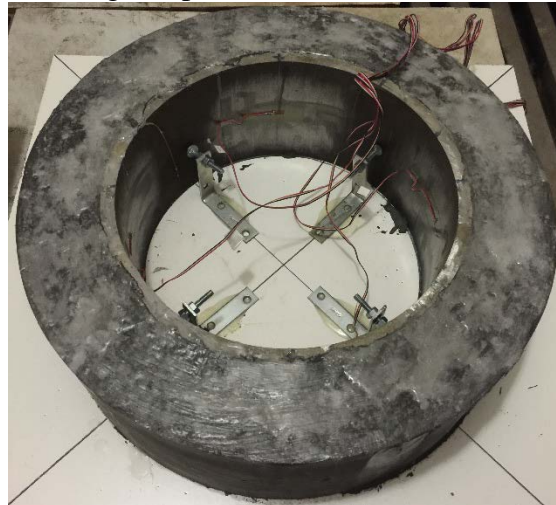
(c) Demolding after 1 day and coating the top surface with paraffin wax
