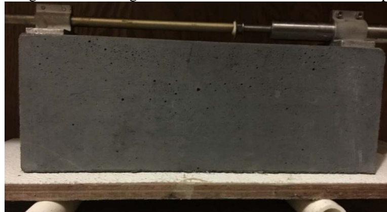
(b) Free Shrinkage Test of 4 inch x 4 inch x 11.25 inch prism
