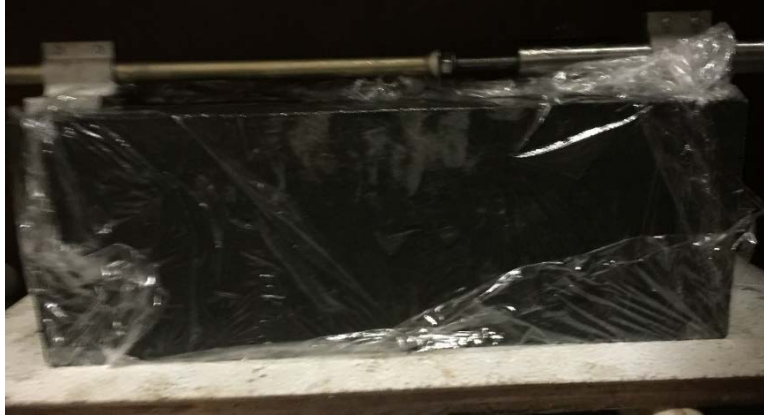
(a) Autogenous Shrinkage Test of 4 inch x 4 inch x 11.25 inch prism
