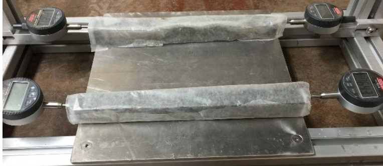
(c) Autogenous Shrinkage Test of 1 inch x 1 inch x 11.25 inch prism
