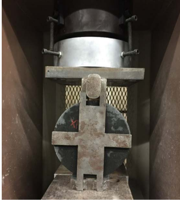
Figure 4.5 Splitting tensile strength test of UHPC (6 inch \times 12 inch cylinder)
