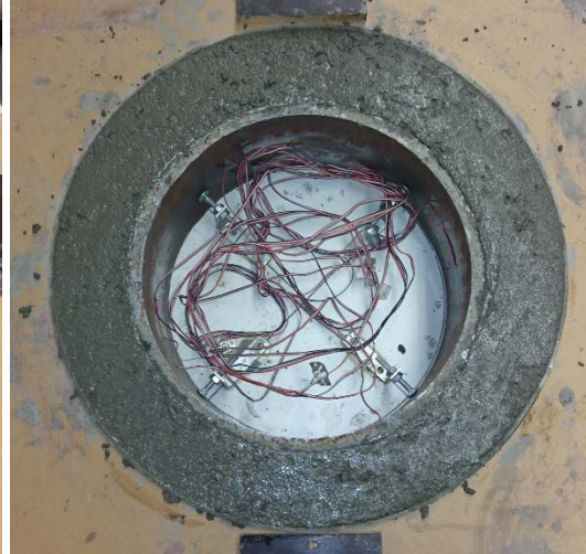
(b) After casting with shotcrete
