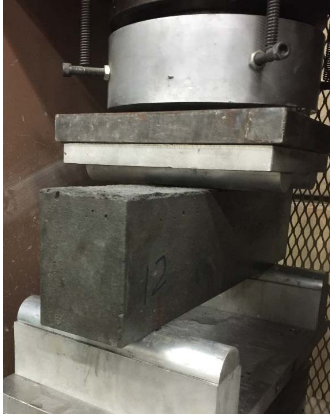
Figure 3.5 Flexural strength test (3 inch \times 4 inch \times 16 inch prism, span: 12 inch)
