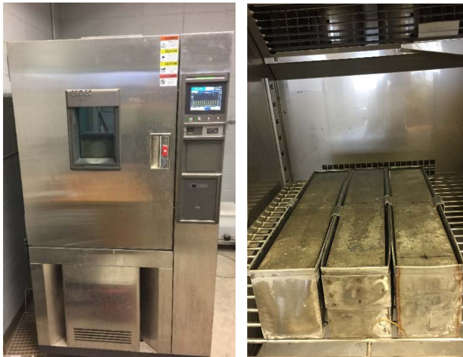
Figure 3.8 Freeze-thaw conditioning chamber
