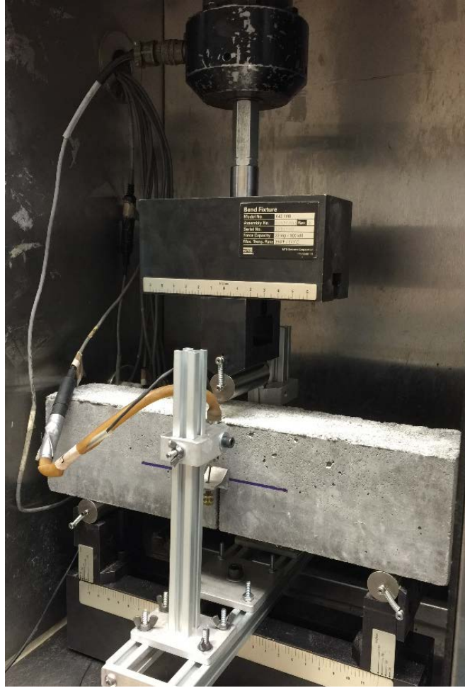
Figure 3.11 Testing equipment setup for fracture test
