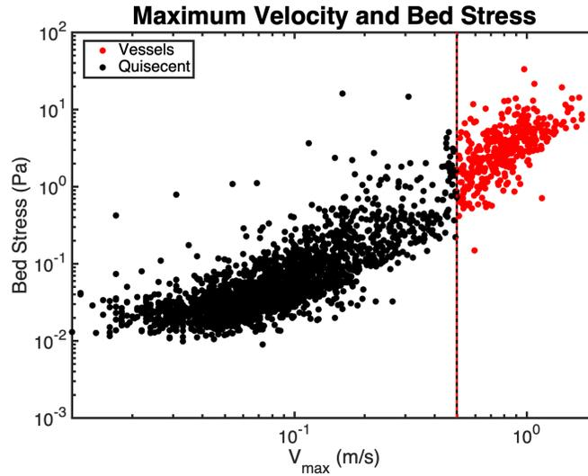
Figure 4: Maximum filtered velocity and bed stress at the south piling of Slip 1 for full vessel arrivals and departures (red), partial arrivals and departures below the maximum velocity threshold (grey) and quiescent periods (black). The dotted black and red line indicates the 50 cm/s threshold for arrival and departure identification.
