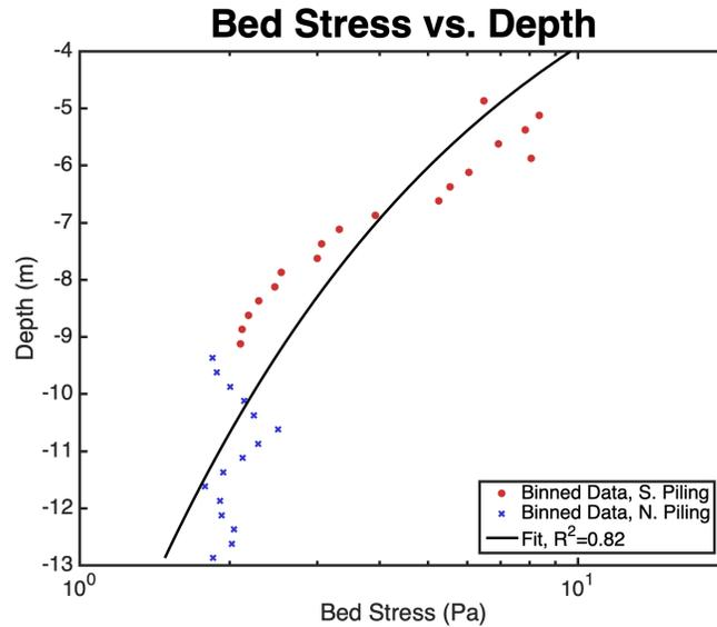
Figure 9: Profiles of bed stress at varying depths for departures at Slip 1. The binned data is shown as colored points (red crosses for the north piling, blue circles for the south) and the fit is shown as a solid black line with an  $R^2$  value given in the legend.
