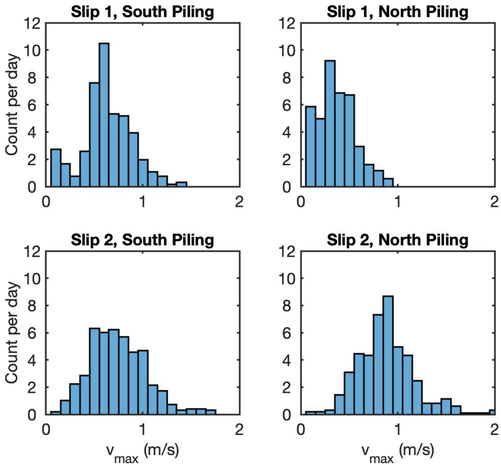
Figure 5: Histograms of maximum velocity during vessel arrivals and departures for each slip and piling. The histograms are normalized such that the y-axis indicates the daily frequency of each 0.1 m/s velocity bin.
