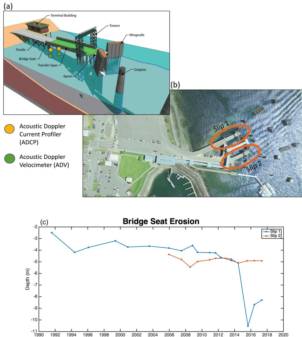
Figure 1: Experimental setup & bed elevation time series at Kingston ferry terminal, WA.
