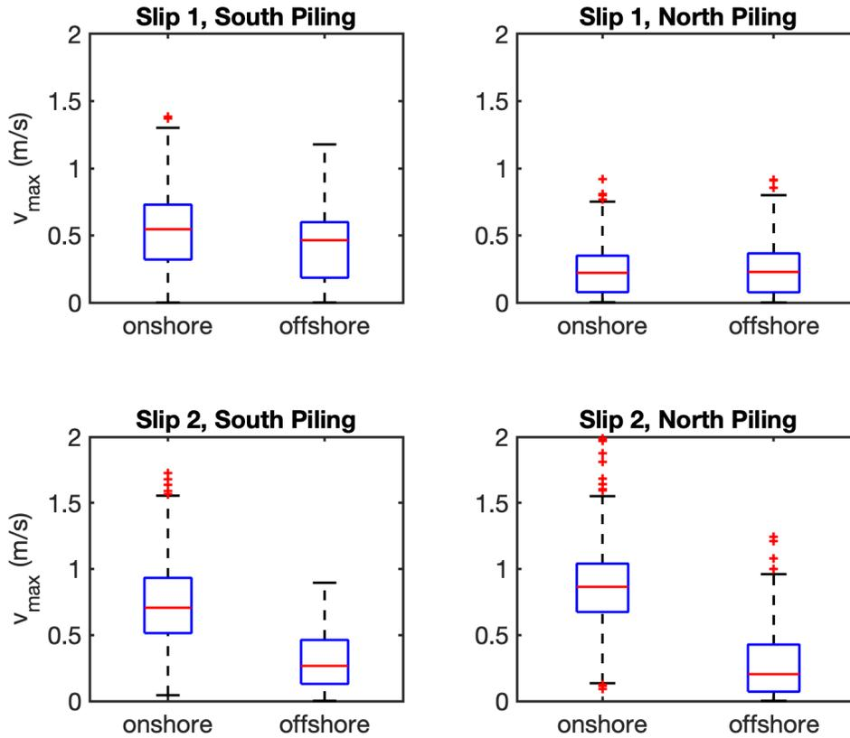
Figure 7: Box plots of onshore and offshore maximum velocity for all vessel arrivals and departures at each slip and piling. The red line in the middle of each box shows the median, while the interquartile range is shown by the box edges. The whiskers indicate an extreme value, and red crosses above the whiskers indicate outliers. Outliers are determined by the Matlab *boxplot* function. Note that infrequent velocities above 2 m/s have not been shown.
