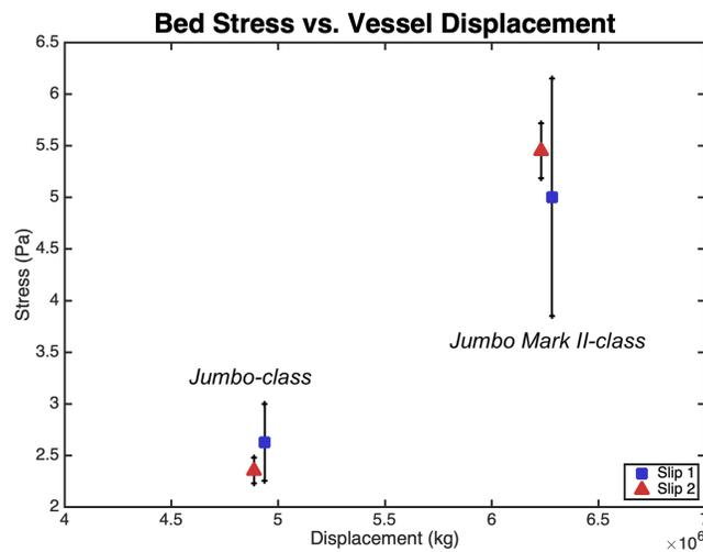
**Figure 10: Bed stress by vessel displacement, averaged over both pilings at each slip.** Slip 1 values are shown by blue squares, Slip 2 values by red triangles. Whiskers show standard error bounds. Each vessel in a vessel class has the same displacement. The apparent small difference in displacement between slips is for legibility only and does not reflect actual differences in vessel displacement.
