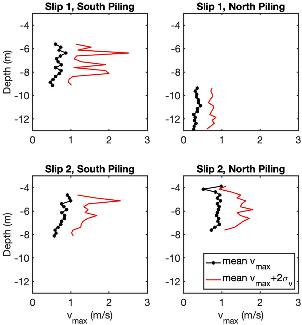
Figure 6: Profiles of the mean maximum velocity in 0.25 m steps of tidally varying depth bins at each slip and piling are shown in black. An upper limit for maximum velocity is given by the red line, which shows the velocity two standard deviations above the mean for a given bin.
