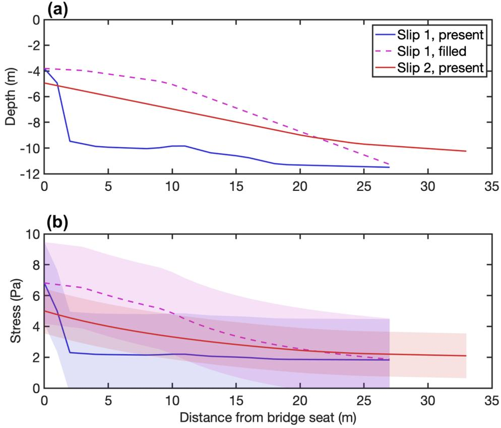
Figure 13: Along-slip profiles of (a) ground line, for Slip 1 (current and proposed) and Slip 2, and (b) stress at the groundline calculated using the model from section . Shaded error bars indicate one half of the standard deviation of stress (mean of the two pilings) observed at each slip.
