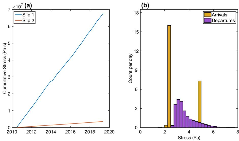
Figure 12: (a) Prediction of cumulative stress for the years 2010-2019 using the model and trends in this report (blue indicates Slip 1, red indicates Slip 2); (b) Histograms of the predicted stress for arrivals and departures, normalized into a daily frequency of each 0.25 Pa stress bin.
