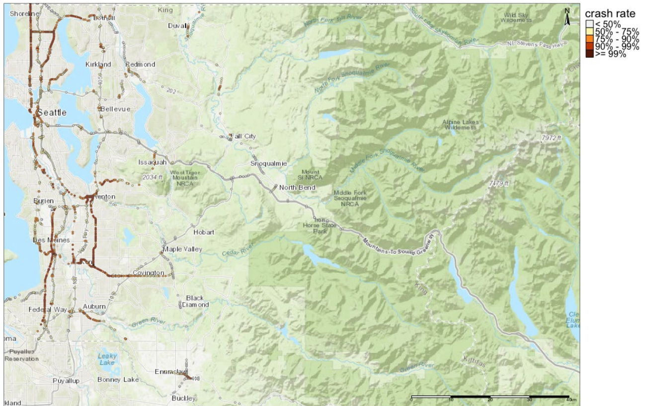
Figure C-1. Map of expected crash frequencies per 100-meter Euclidean buffer of pedestrian-vehicle crashes at intersection and non-intersection locations along the state routes in King County
