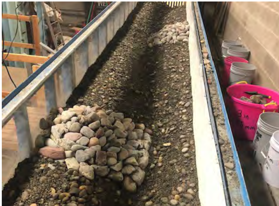
Figure 13 Construction of boulder bars spaced three channel widths apart.
