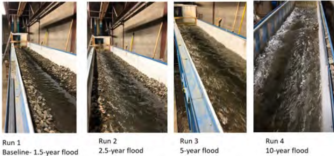
Figure 5 Shows each flood event in the study section. The figure on the far left shows the channel during run 1. The middle figure shows the flow in the channel during run 2. The flow has filled the U-shape channel. The figure on the right is run 3 in the channel. This final run has submerged the whole channel and extends up the side of the flume.
