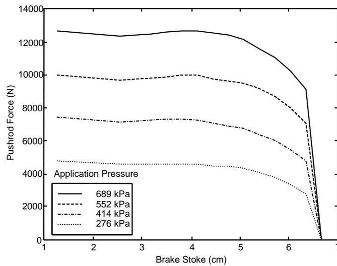
**FIGURE 3 Measured Effect of Brake Stroke on Pushrod Force.**
