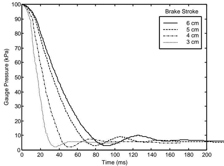
**FIGURE 9 Air Pressure Decay from Air Brake Chamber Model.**
