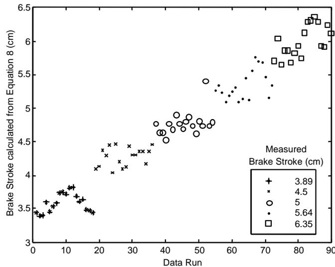
**FIGURE 11 Comparison of Measured and Determined Brake Stroke.**
