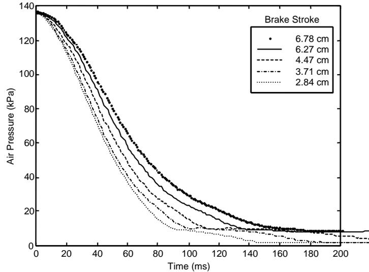
**FIGURE 10 Experimental Air Pressure Decay Data.**
