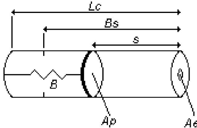
**FIGURE 4 Simplified Air Brake Chamber Geometry.**
