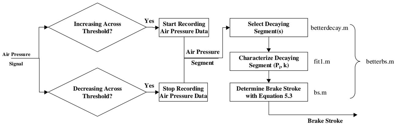
FIGURE 13 Air Pressure Analysis Block Algorithm.
