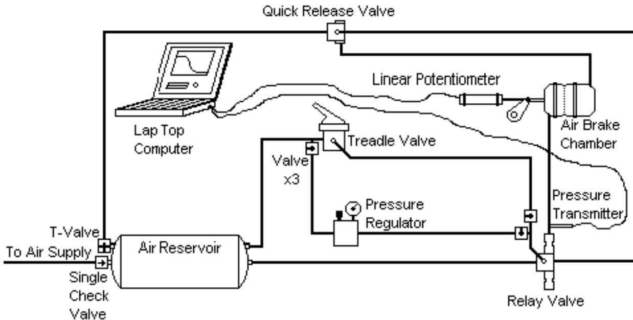
**FIGURE 5 Schematic of Laboratory Setup.**
