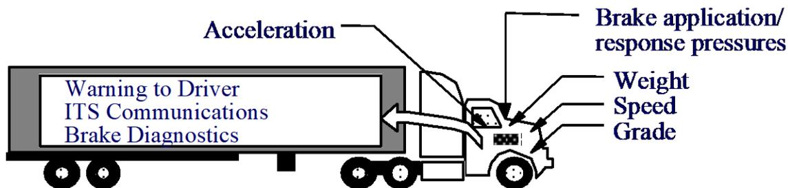
FIGURE 1 Brake Condition Monitoring System Concept.
