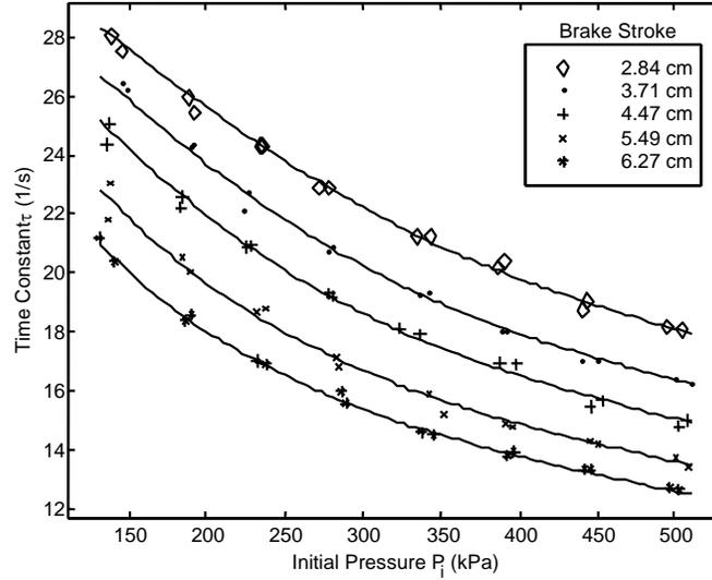
**FIGURE 7 Correlation between  $P_i$ ,  $\tau$ , and Brake Stroke.**
