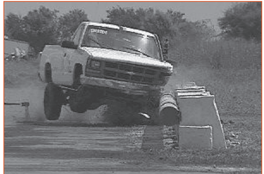
A new roadside barrier was designed and tested for use in locations where historical context or aesthetics are a concern.
