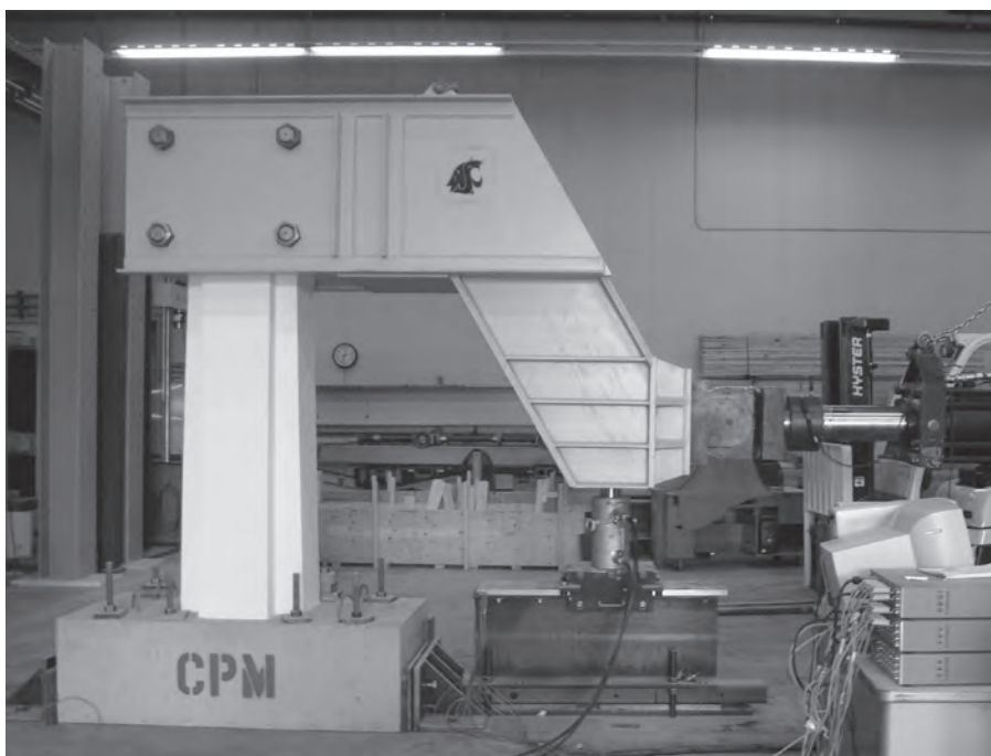
Columns from the Aurora Avenue Bridge are tested at Washington State University. (Photo provided by David McLean)
