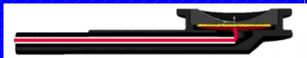
Figure 3: Diagram of electrical connections in the transducer. Grey represents ground and represents positive, white represents black, and yellow represents the crystal.
