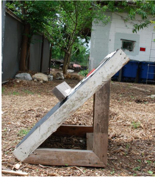
Figure 10. UV Disinfection structure
