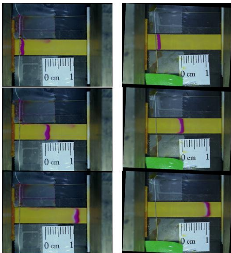
Figure 4. Sequence of frames containing band markers travelling from left to right in two different devices (left and right columns, respectively) showing varied band morphology due to differences in electrode contact. The leading and trailing edges of marks develop different curvatures. The white-colored region trailing the markers, which becomes more prominent in the bottom frames, is discussed in the “Aim II” section of the results.
