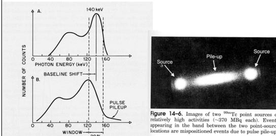
Fig. 11-10. (A) <sup>99m</sup>Tc spectrum at low counting rate. (B) Spectral broadening and shift in apparent photopeak energy due to pulse pile-up and baseline shift in the spectrometer amplifier at high counting rate.
