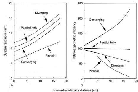
**Figure 14-21.** Performance characteristics (A, system resolution; B, point-source geometric efficiency in air) versus source-to-collimator distance for four different types of gamma camera collimators. (Reprinted by permission of the Society of Nuclear Medicine from Moyer RA: A low-energy multihole converging collimator compared with a pinhole collimator. J Nucl Med 15:59-64, 1974.)
