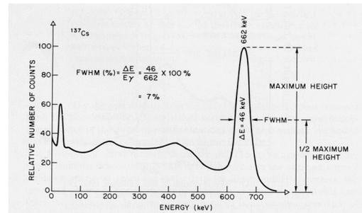
**Fig. 11-11.** Calculation of FWHM energy resolution of a NaI(Tl) detector for <sup>137</sup>Cs 662 keV  $\gamma$  rays.
