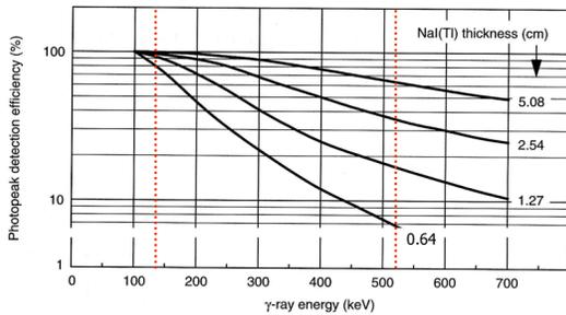
**Figure 14-3.** Photopeak detection efficiency versus  $\gamma$ -ray energy for NaI(Tl) detectors of different thicknesses. (Adapted from Anger HO: Radioisotope cameras. In Hine GJ [ed]: Instrumentation in Nuclear Medicine, Vol 1. New York, Academic Press, 1967, p 506.)
