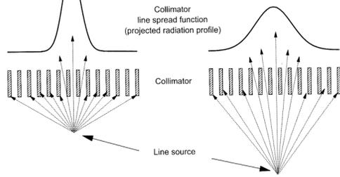
**FIGURE 21-12.** Line spread function (LSF) of a parallel-hole collimator as a function of source-to-collimator distance. The full-width-at-half-maximum (FWHM) of the LSF increases linearly with distance from the source to the collimator; however, the total area under the LSF (photon fluence through the collimator) decreases very little with source to collimator distance. (In both figures, the line source is seen "end-on.")
