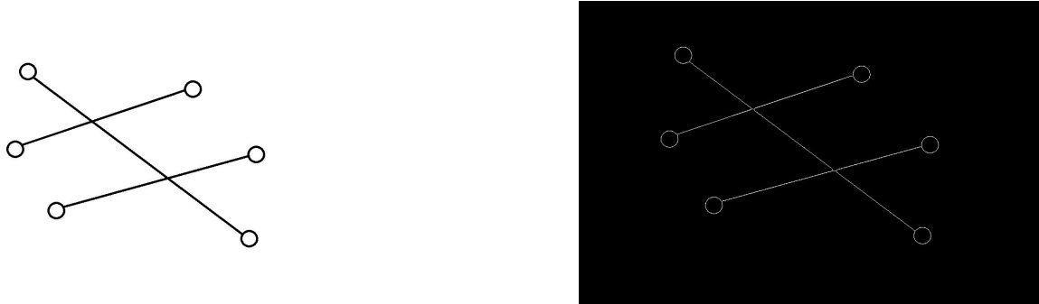
Fig. GR01 The left one is the original image while the right one is the binary thinned version.
