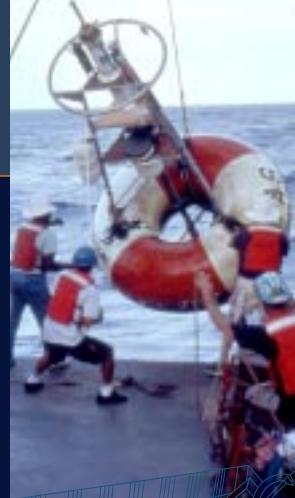
Deployment of a buoy in an array of moorings that measures winds; air, sea-surface, and subsurface temperatures; relative humidity; and ocean currents (TAO project of NOAA/PMEL)
