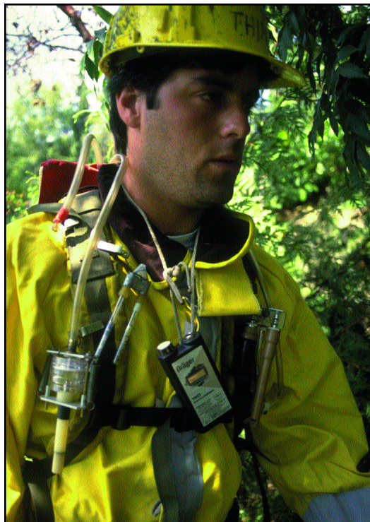
Figure 1—Smoke exposure sampling apparatus.
