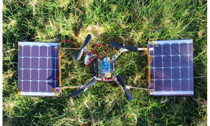
Fig. 1: The palm-sized drone carries two lightweight solar panels, a maximum-power-point tracking charging circuit, and a sensor package that allows it to fly autonomously and detect suitable sites for charging.
