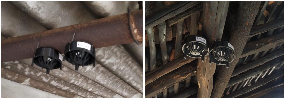
Figure A5. Deployment of paired low-cost passive samplers side-by-side in two indoor locations hanging from (left) a metal ceiling and (right) a wood ceiling.
