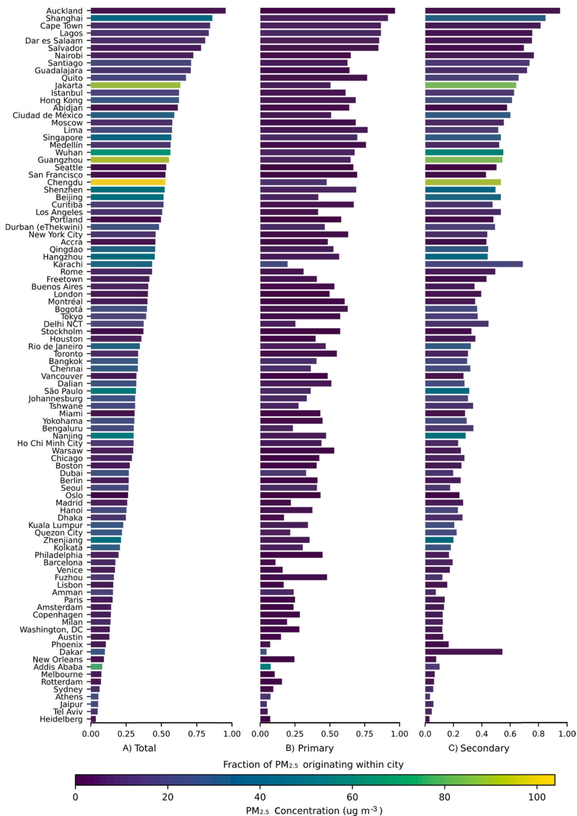
Fig. 1. Fractions of PM 2.5 originating from within city sources for A) total PM 2.5 , B) primary PM 2.5 and C) secondary PM 2.5 among 96 global cities. Color scales represent population-weighted PM 2.5 concentration ( \mu\text{g m}^{-3} ). (For interpretation of the references to colour in this figure legend, the reader is referred to the Web version of this article.)
