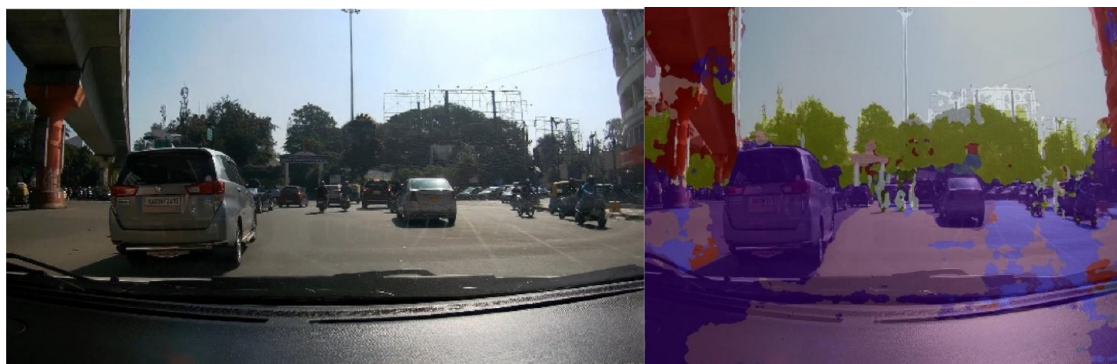
Figure 4. Semantic segmentation: the original frame appears on the left, and the pixel labeling by category on the right.
