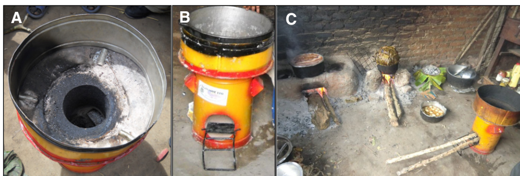
Fig. 2. The wood-fueled rocket stove (Ugastove) used in this intervention (A & B). Three types of stoves present in each study village (C) from left to right: locally produced clay and anthill dirt stove, three stone fire, and the Ugastove.
