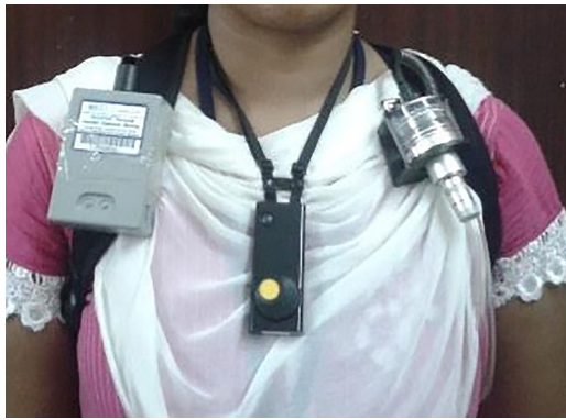
Fig. 5. Personal monitoring equipment used in panel study including (from left to right) MicroPEM, wearable camera, and gravimetric sampler.
