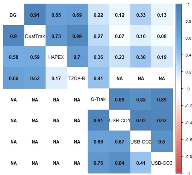
Fig. 1. Correlation (above the diagonal) and concordance (below the diagonal) matrices between the low-cost devices and the benchmark monitors used in the experiment in Spain. BGI and DustTrak DRX: benchmark PM 2.5 monitors; HAPEX and TZOA-R: low-cost PM 2.5 monitors; Q-Trak: benchmark CO monitor; (EL-)USB-CO: low-cost CO monitor. The number at the end of each (EL-)USB-CO indicates a different unit of the same device. To obtain both matrices, PM 2.5 data from the 5 sampling days was used for all monitors except for TZOA-R, for which only data from the two last sampling days was obtained. To obtain both matrices, CO data from the last two sampling days was omitted due to monitor malfunctioning. The “NA” in the case of TZOA-R correlations means that no simultaneous and valid data are available for both devices. Note that correlation and agreement for BGI pairs were averaged over 4 h for daytime / 8 h for night time. All other data in Figure are based on 5 min averages. DustTrak DRX, HAPEX, and TZOA-R data presented here are adjusted gravimetrically and by relative humidity. Colour legend bar at the right indicates the magnitude of the correlation and agreement from -1 to 1; lighter cells indicate proximity to 0.
