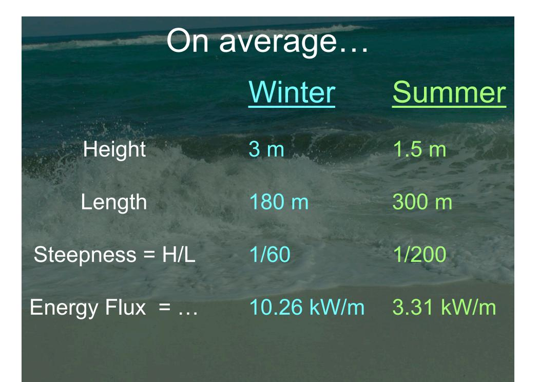
Wint Summ **Energy Flux** Height er er Length  $= c_g (KE+PE)$ 3 m 1.5 m Steepne 180 300 m 1/200 SS m Group Velocity = 1/2 (Phase Speed in Deep Water)  $= \frac{1}{2} (gL/2\pi)^{\frac{1}{2}}$ WINTER: 8.38 m/s SUMMER: 10.82 m/s
