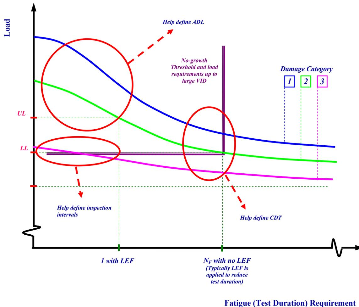
Figure 4. Application of LLD hybrid approach for full-scale demonstration.
