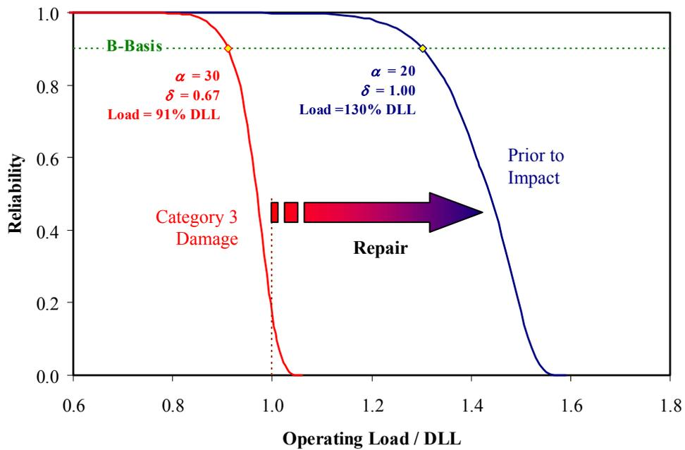
Figure 8. Static-strength reliability comparison before and after impact.
