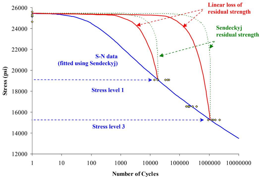
Figure 9. Residual strength degradation for constant amplitude fatigue loading.
