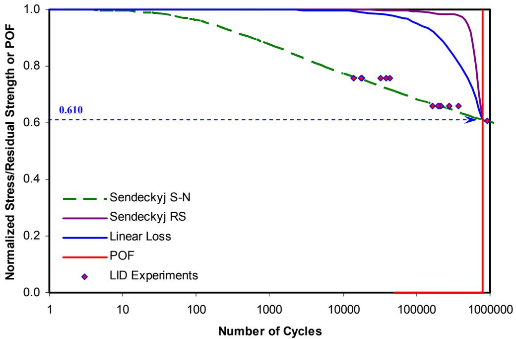
Figure 11. Example of CFU model for constant amplitude fatigue tests.
