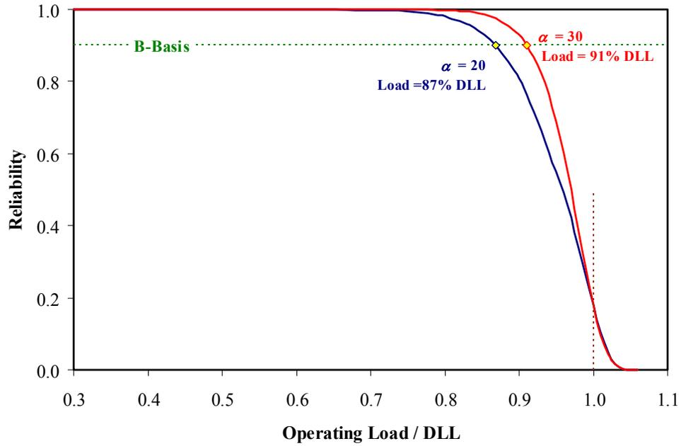
Figure 7. Static-strength reliability at operating loads for a structure with a category 3 damage.
