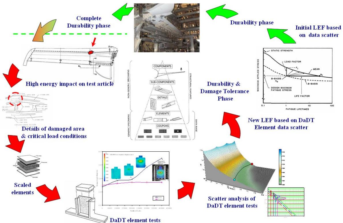
Figure 2. DaDT test demonstration with Load-Life-Damage hybrid approach [4].
