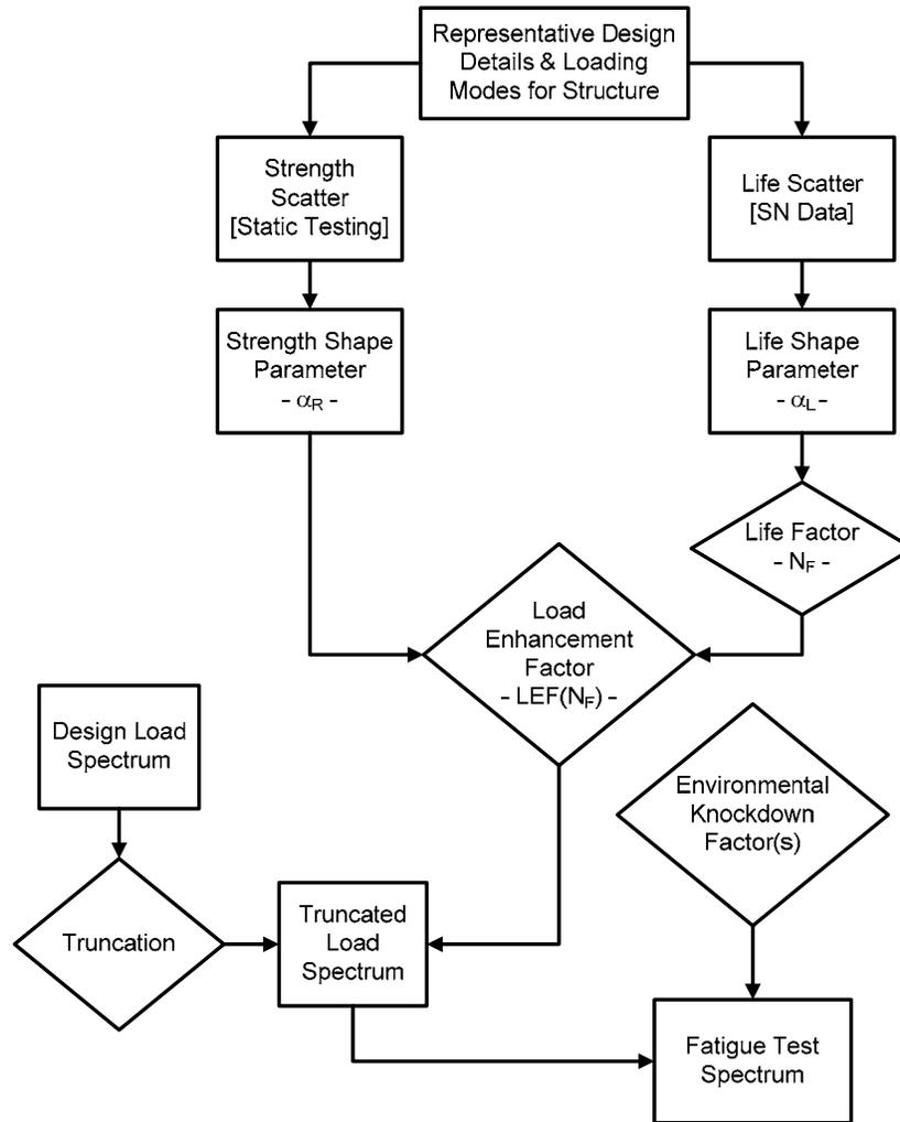
Figure 1. Derivation and application of life and load-enhancement factors through scatter analysis of composite test data.
