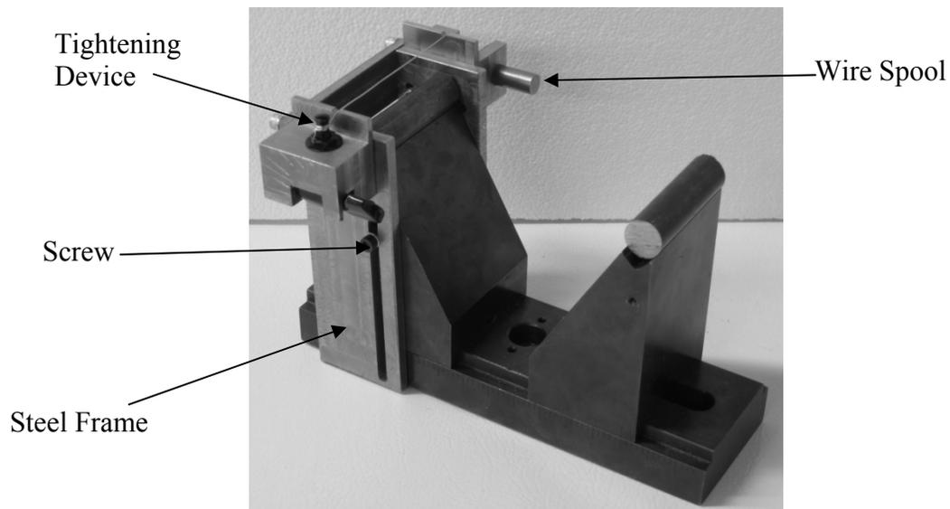
FIGURE 6: PROTOTYPE END NOTCHED SHEAR TEST FIXTURE
