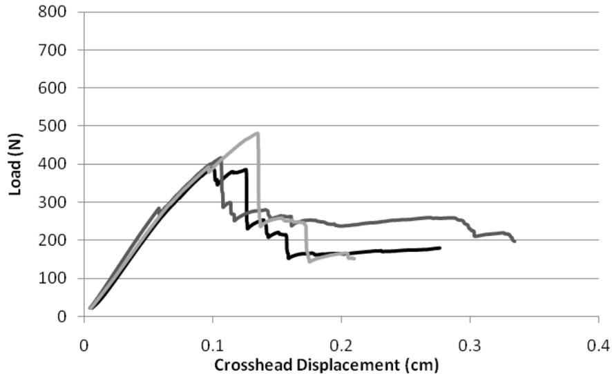
FIGURE 7: REPRESENTATIVE LOAD-DISPLACEMENT CURVES FROM MODE II TESTING OF NOMEX HONEYCOMB CORE SPECIMENS
