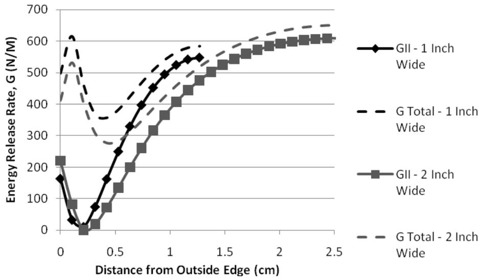
FIGURE 8: ENERGY RELEASE RATE VS. DISTANCE FROM SPECIMEN EDGE
