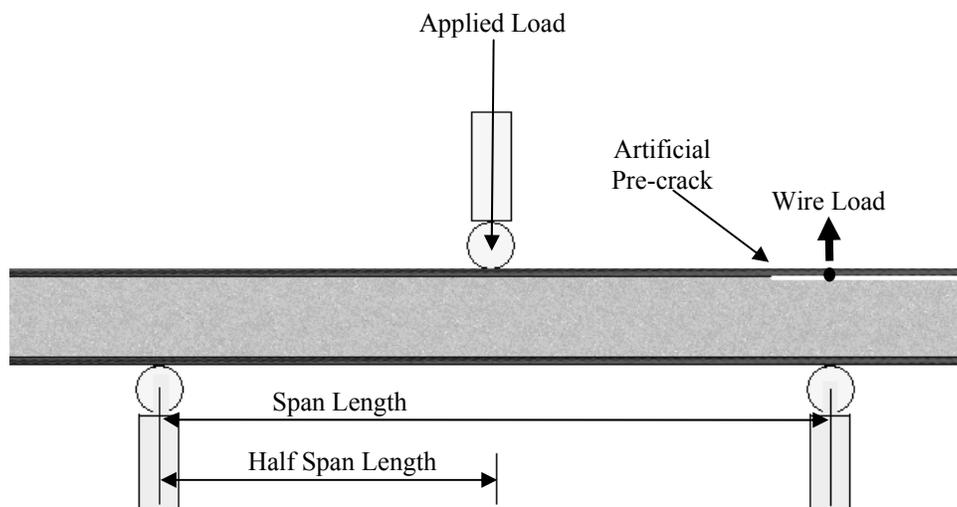
FIGURE 5. END NOTCHED SHEAR TEST
