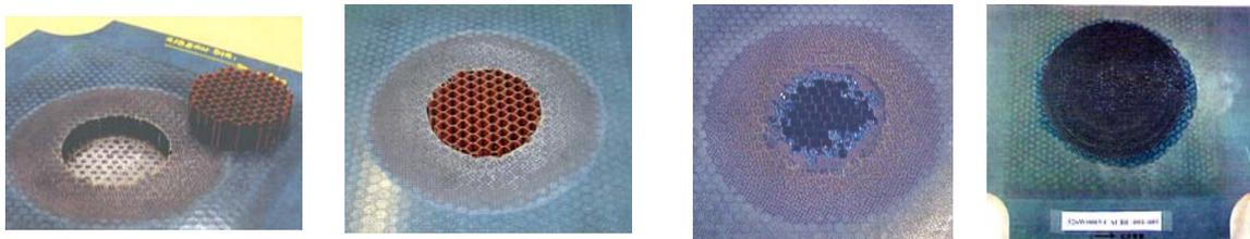
Figure 4. Picture Frame shear elements repaired using the CACRC method
