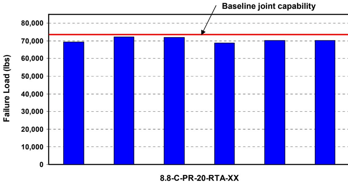
Figure 8. Ultimate Strength of PR (perspiration) Contaminated Specimens
