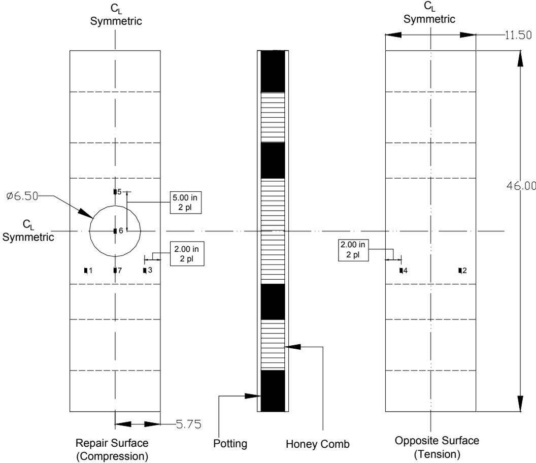
Figure 12. Specimen Instrumentation
