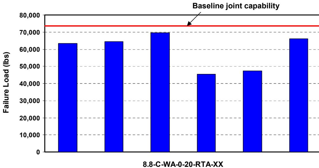
Figure 7. Ultimate Strength of WA-0 Contaminated Specimens
