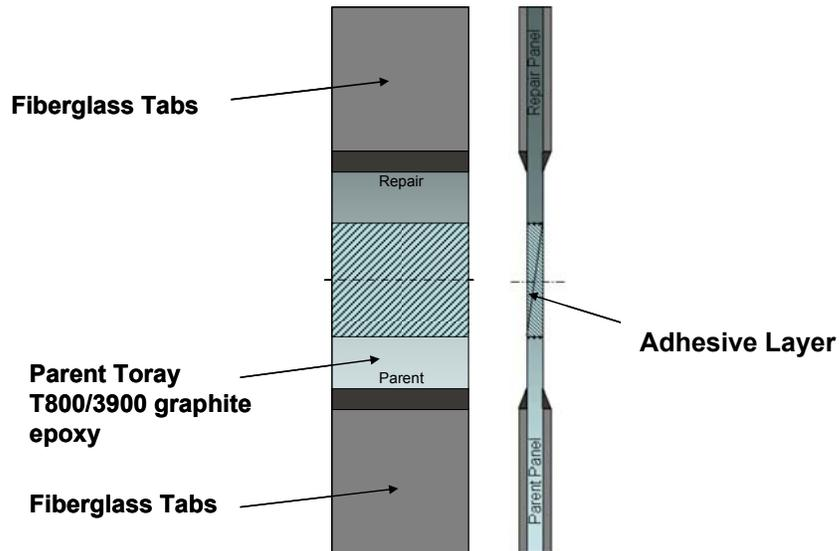
Figure 5. Laminate Scarf Joint Configuration
