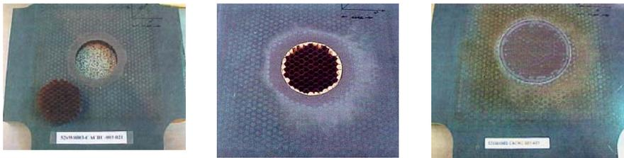
Figure 3. Picture Frame shear elements repaired using the OEM method
