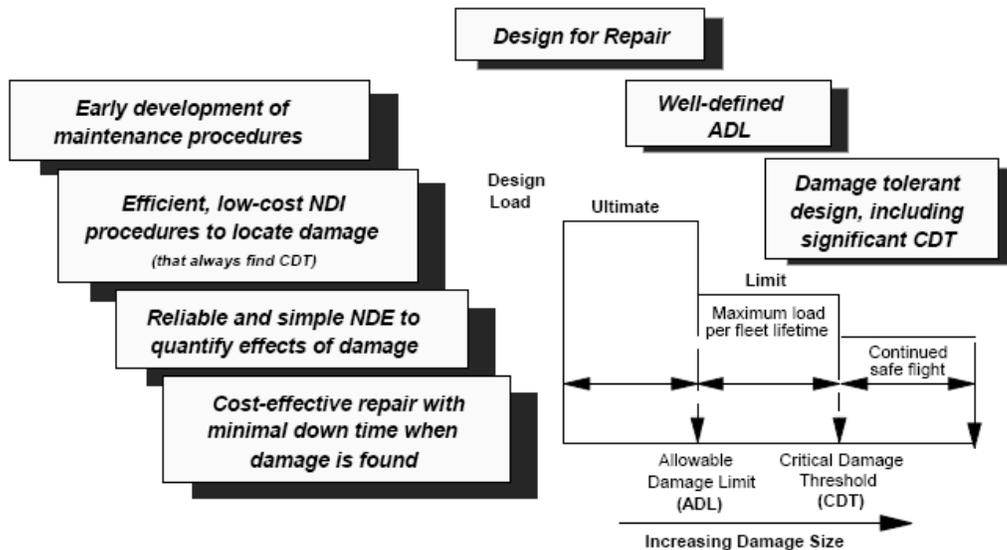
Figure 1. Maintenance development philosophy established during the Boeing/NASA (ATCAS) composite fuselage program
