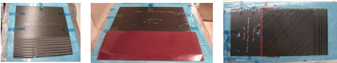
Figure 6. Scarfed laminate preparation and repair procedure
