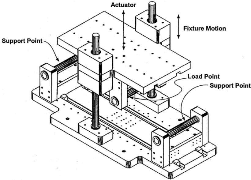
Figure 11. Isometric view of test fixture.
