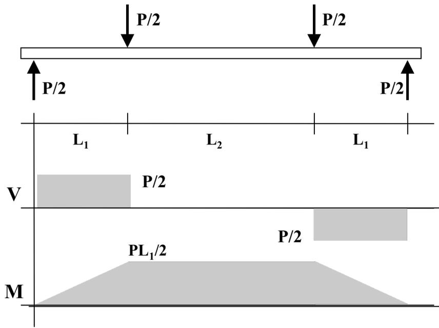
Figure 2. Shear and bending moment diagram for four point flexure test.
