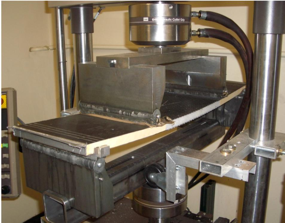
Figure 3. Four point flexure test fixture used for assessing damage tolerance of sandwich composites at the University of Utah.
