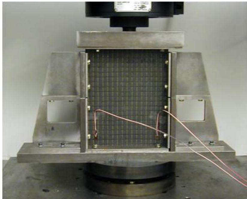
Figure 1. Compression After Impact (CAI) test fixture for composite sandwich panels used at the University of Utah.
