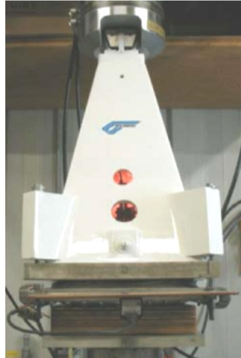
Figure 4. ASTM D6416 “Hydromat” sandwich panel test configuration [10].
