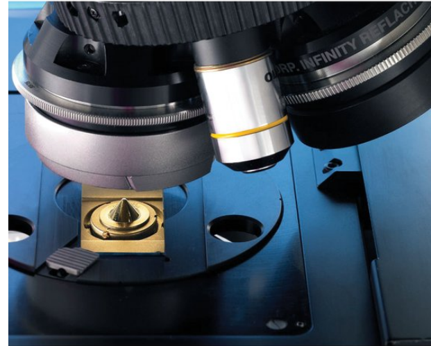
Spatial resolution achievable with the Slide-On TipATR Objective (Photomask target. Lateral profile <math>< 5 \mu\text{m}</math> wide)
