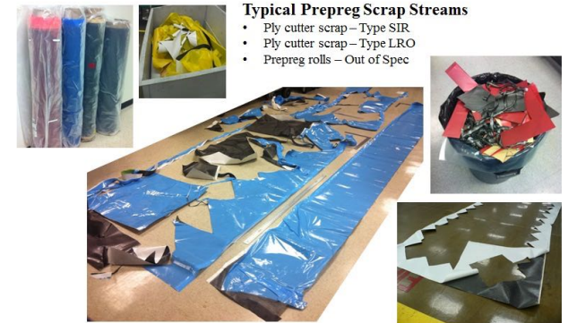
Ply Cutter Scrap Classification Legend Char 1: S=small, M=medium, L=large; Char 2: I=irregular, R=regular; Char 3: R=random, O=ordered
