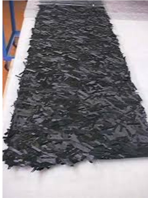
HexMC Material, (450mm wide Roll), ~2000 gsm, ~2 mm thick
