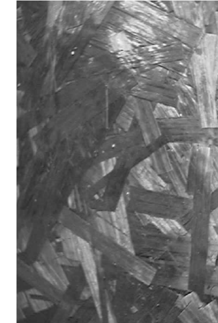
50mm x 8mm 8552/AS4 UD 150 gsm, 38% RC, Controlled Random Distribution
