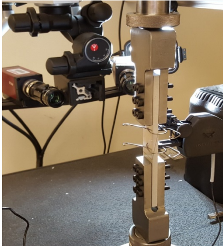
Cyclic testing of scarf joint on an Instron to quantify adhesive hardening
