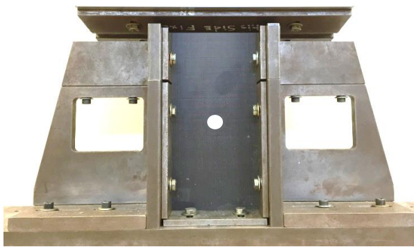
Sandwich Open Hole Compression
