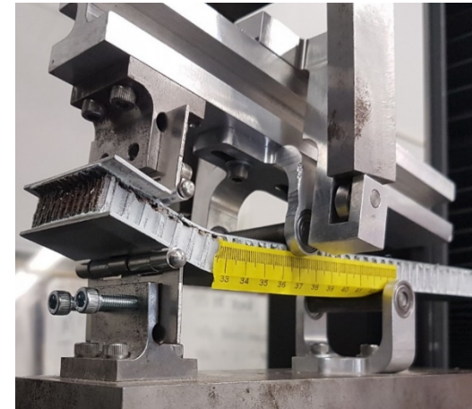
Sandwich Mixed Mode Bend Test
