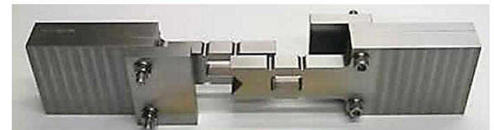
Open hole compression fixture for monolithic composites
