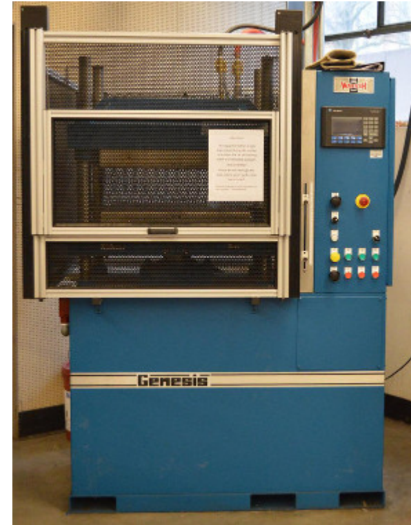
Wabash Model G50H-24- BCLX 50-ton hot press
