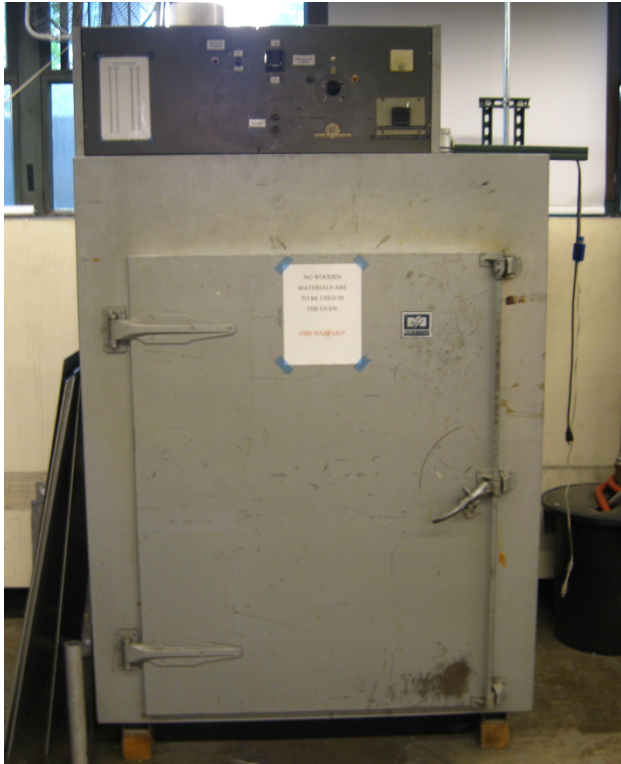
Blue-M Model POM-246F Lab Oven
