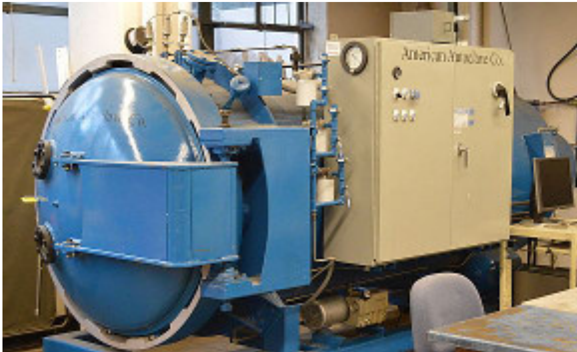
American Autoclave featuring 42 in dia x 96 in working chamber
