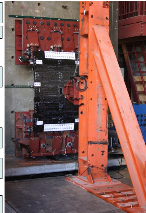
1D Dynamic Shake Table. Impactor head moves into specimen – simulating GSE contact.
