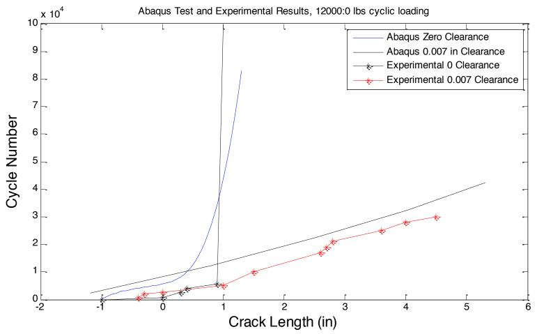
Fatigue model and test results agree better when identical (quasi-isotropic) layup used for fatigue properties
