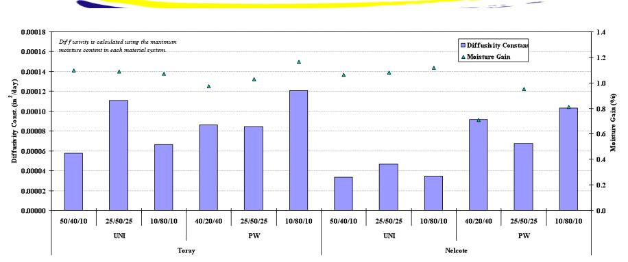
Diffusivity was calculated using the maximum moisture content (per AGATE criterion) in **each material system**.
