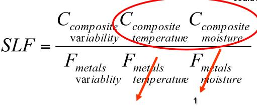
Room for improvement in this based upon failure mode in temperature (based upon FEM M.S. model) and amount of moisture actually expected in structure during lifetime
