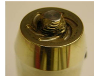
Figure 3. Tool designs include the classic TWI 5651, Tri-flute™, Scrolled shoulder with threaded pin and straight flats, Small (shoulder) Wiper™ with threaded pin and twisted flats, and a Wiper™ (large diameter shoulder) with threaded pin and twisted flats. [1,12]
