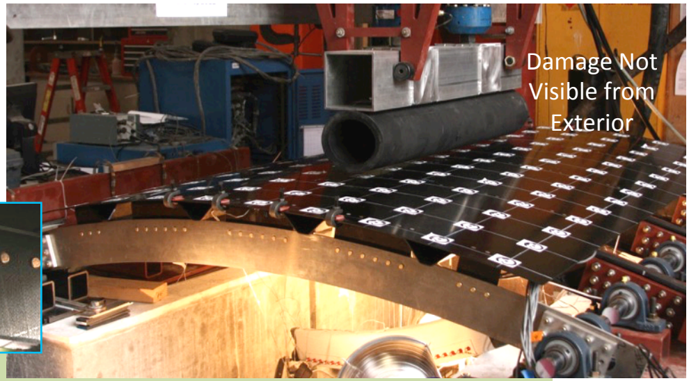
Frame Failure Near Outer Shear Ties
